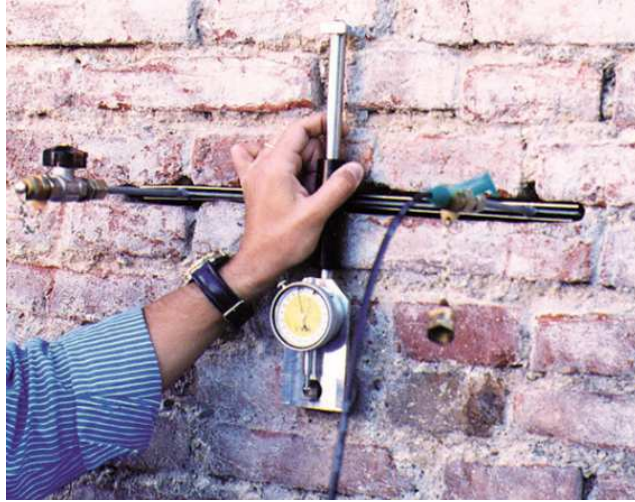
Fig. 1.16 Image of a flat-jack test
