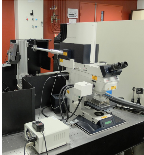
Fig. 1.8 – Confocal microscope Leica TCS SP2 SE form Hubert Curien Laboratory (Saint-Étienne, France)
