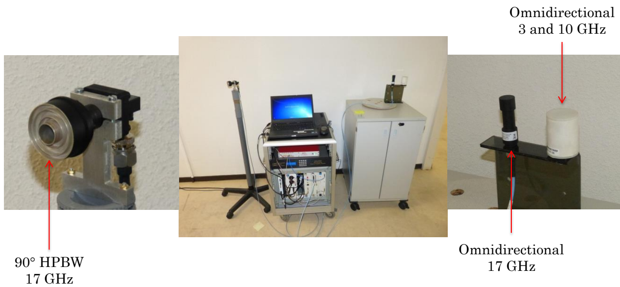
Fig. IV.1.4 – RX/MS measurement equipment (1)
