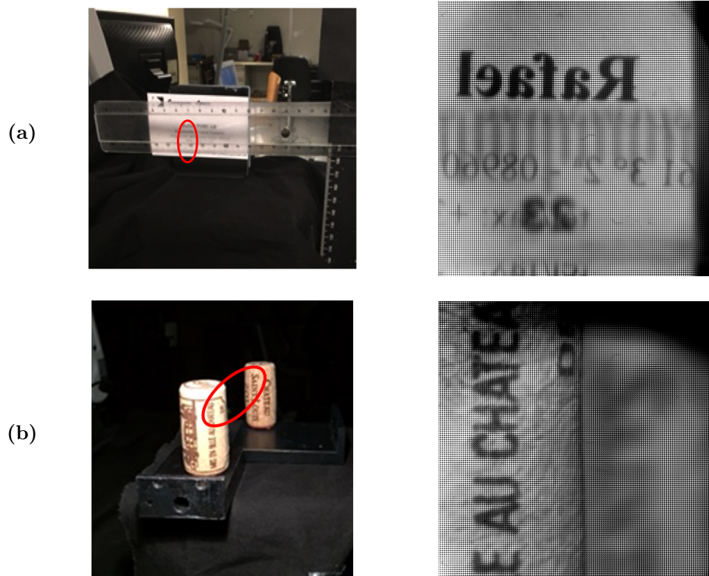
Figure 4.9: On the left column, some test objects photographed by a mobile camera. The red circle superimposed to the images shows the restricted field of view recorded by our plenoptic camera. On the right column, the light field images taken with our plenoptic camera prototype.
