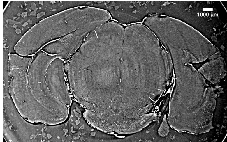
Figure 2.14: 2D XPCT coronal image of the healthy brain sample selected at mid-depth of the brain.
