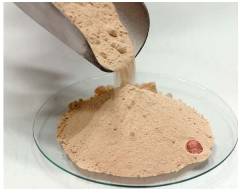
Figure I-16. Gypse synthétique issu du procédé FGD (“What are coal combustion by-products (CCBs), Center for applied energy research, University of Kentucky,” n.d.)
