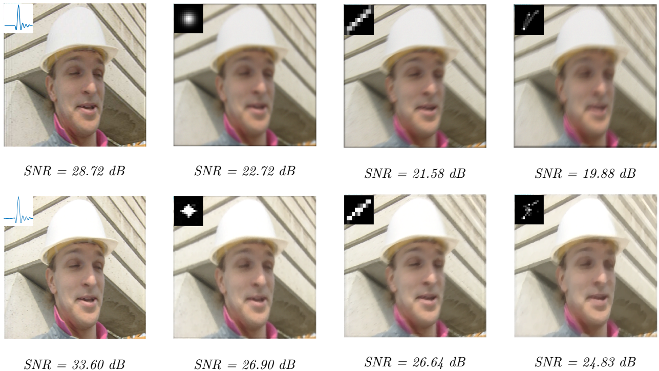
Figure 7.7: Foreman sequence: images from the degraded sequence (top), corresponding restored images with the best choice of spatial regularizations in terms of SNR (bottom).
