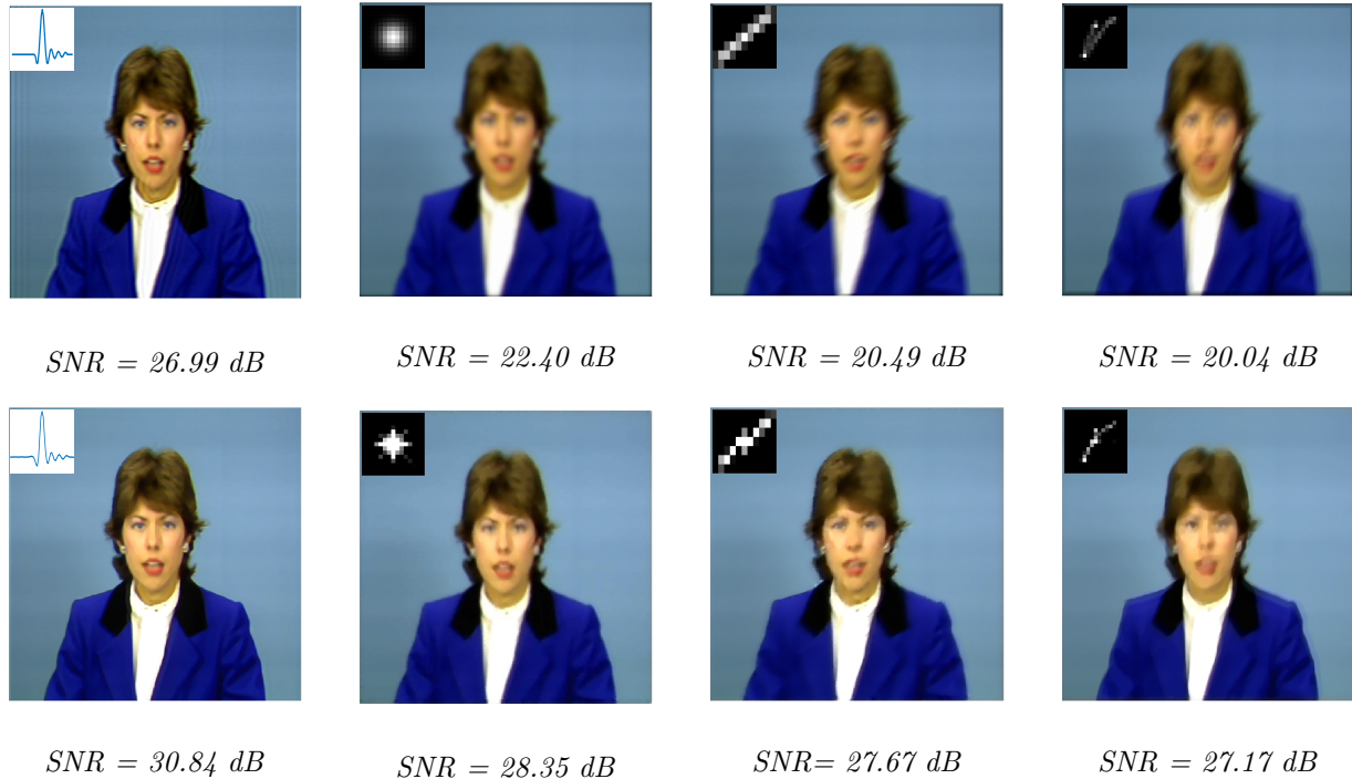
Figure 7.8: Claire sequence: images from the degraded sequence (top), corresponding restored images with the best choice of spatial regularizations in terms of SNR (bottom).
