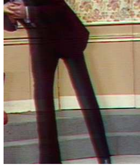
Figure 2.12: Ghost effect that appears as a shadow at the right of the main image.
