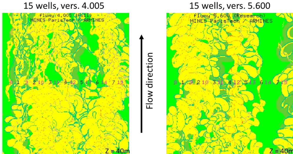
**Figure 135. Comparison of horizontal slices of two simulations: conditional by 15 aligned wells, Flumy vers. 4.005 (left) and conditional by 15 aligned wells, Flumy vers. 5.600 (right). Z = 40m**
