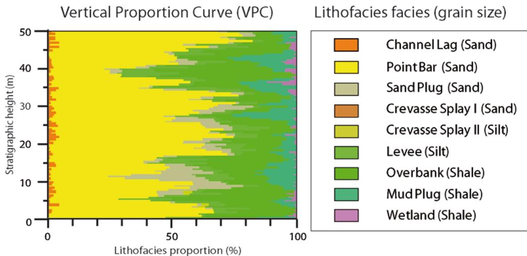
Figure 139. Example of a Vertical Proportion Curve (VPC) with its lithofacies color scale. Image from Flummy<sup>®</sup>
