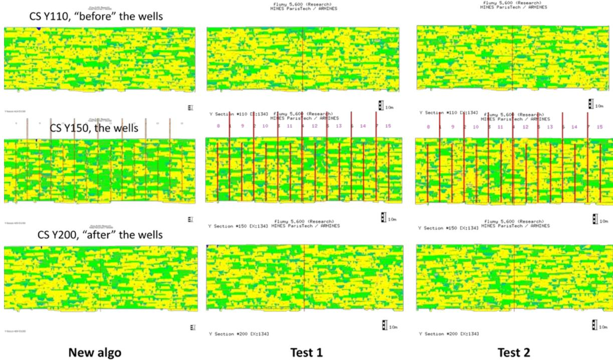
Figure 138. Comparison of vertical model cross-sections before the wells, containing the wells and after the wells, for three models: original vers. 5.600, vers. 5.600 without migration repulsion for OB/LV reproduction and vers. 5.600 without migration repulsion at all
