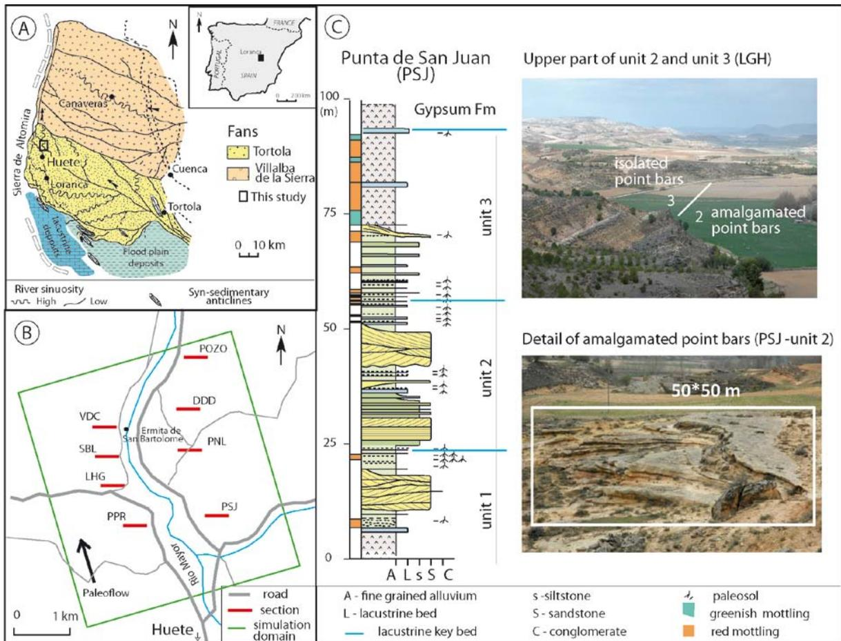
**Figure 142.** Loranca basin: (a) location of the study area in the Tortola fan and (b) location of the measured sections along the Rio Mayor valley sides with (c) an illustration of the architecture of isolated and amalgamated sand bodies
