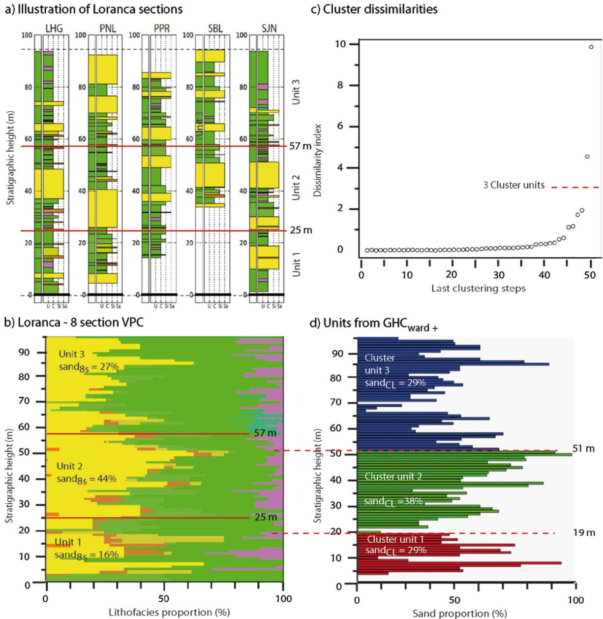
**Figure 146. Application to a real dataset: Loranca basin. (a) 5 sections out of the 8 available, red solid lines represent units limits proposed by geologists. (b) VPC of the 8 Loranca wells. (c) Cluster dissimilarities graph. (d) The last three clusters proposed by our method**
