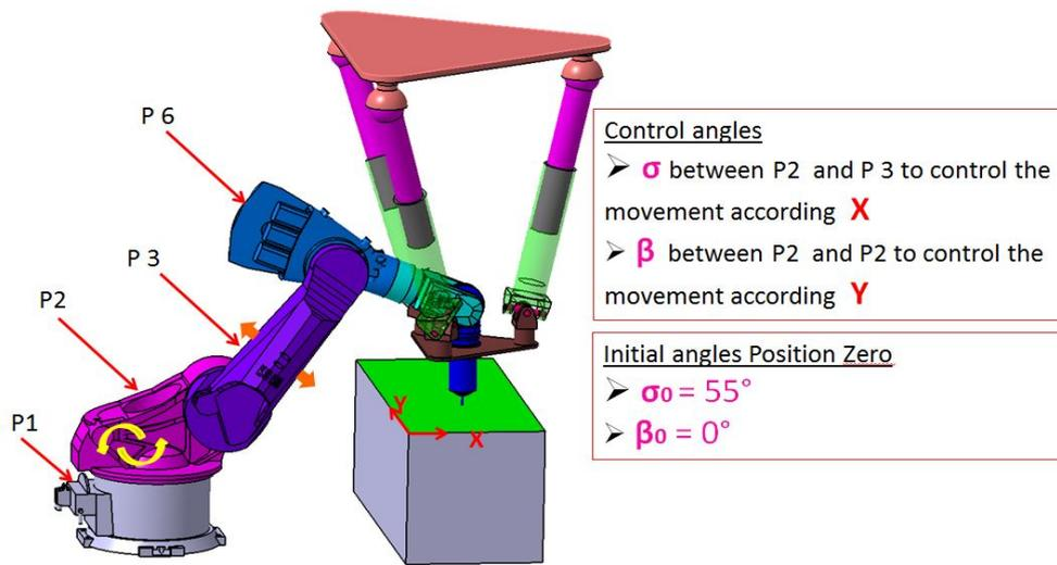
FIGURE 7.37 – Workspace of the hybrid structure
