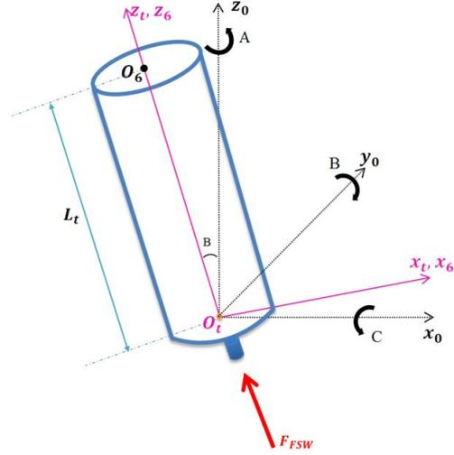
FIGURE 7.3 – Coordinates to define the tool orientation
