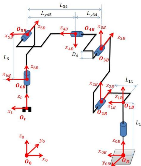
FIGURE 7.15 – The kinematic diagram of the robot B
