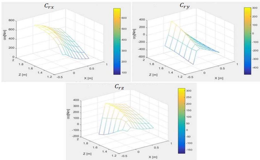
FIGURE 7.27 – Optimal torques created by robot B
