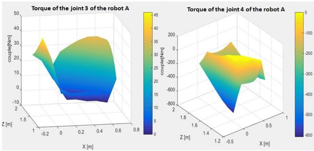
FIGURE 7.29 – Torque of the joints 3 and 4 of the robot A after optimization
