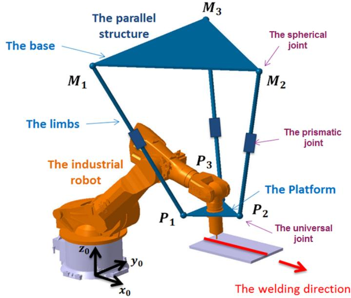
FIGURE 7.2 – Definition of the parallel structure
