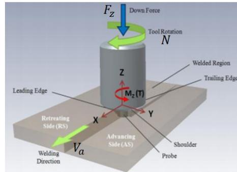
FIGURE 7.1 – Principle of the FSW Process [38]
