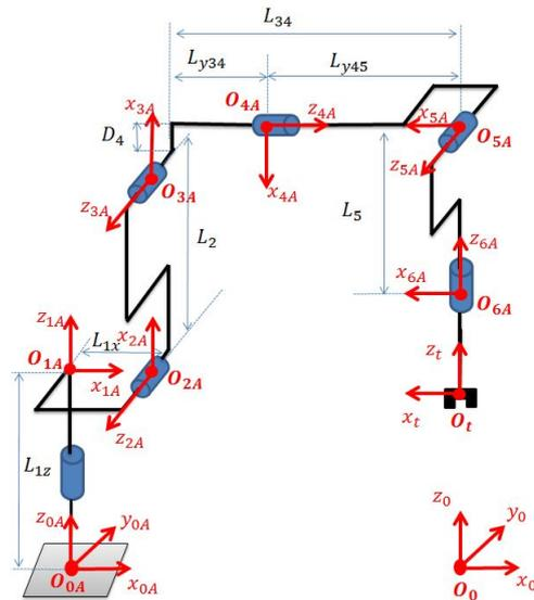
FIGURE 7.14 – The kinematic diagram of the robot A
