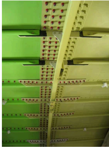
Figure 2.1.1: A typical assembly interface between two fuselage panels involving hundreds of holes.
