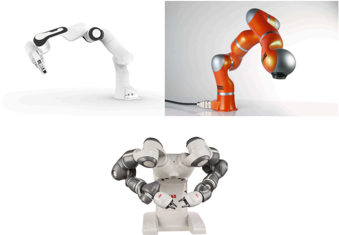
Figure 1.3.3: Other examples of 7 DOFs anthropomorphic arms, and SRS type robots. Collaborative robots Franka Emika Panda, KUKA LWR4 and ABB Yumi.
