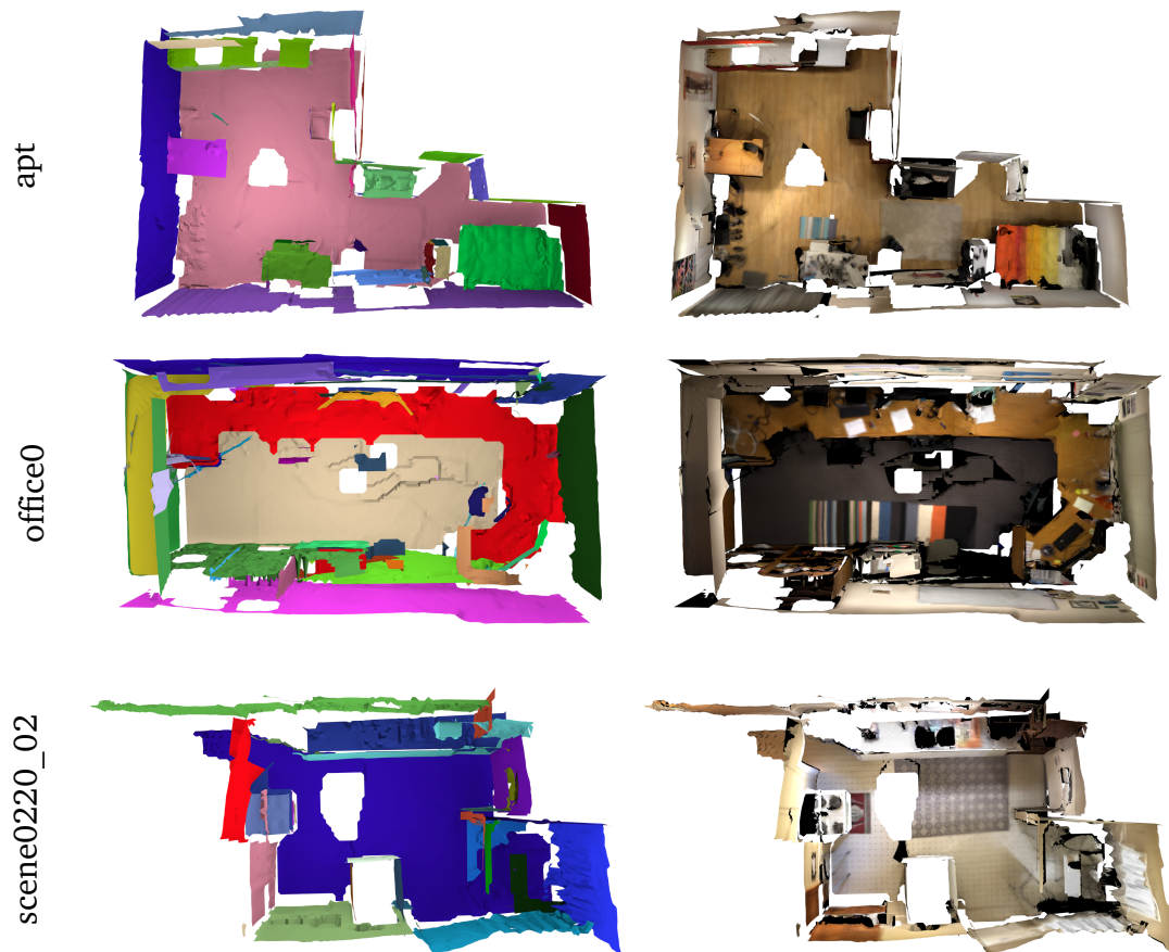
Figure V.5: Examples of reconstructed scenes of the 3DLite [HDGN17] dataset using our geometric proxies. On the left, each proxy is shown with a different random color. On the right, textures have been generated from the color points stored in the proxies (see section IV.3.3). The meshes are made of quads when four activated cells are adjacent, and triangles otherwise.
