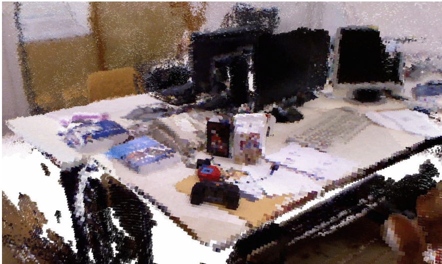
Figure II.10: 3D map built by RGB-D SLAM . Occupied voxels of the fixed 1cm grid are shown with averaged colors. Image taken from Endres et al. [EHS + 14].
