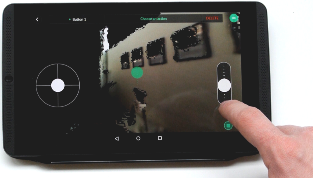
Figure A.2: Geometric proxies in Hayo mobile app. In the 3D viewer of the companion app for the Hayo camera, proxy inliers are replaced by the textured proxy mesh to offer a more complete and intuitive visualization during the process of placing interaction zones (light green sphere). In addition, streaming the compressed proxy version of the data increases the refreshing rate of the 3D information.
