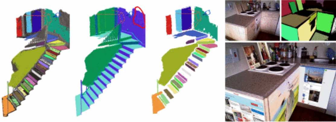
Figure II.11: Planar map creation with dense planar SLAM . The identification of large planar areas in the scene allows augmenting them with web content in real-time. Image taken from Salas-Moreno et al. [SMGKD14a].
