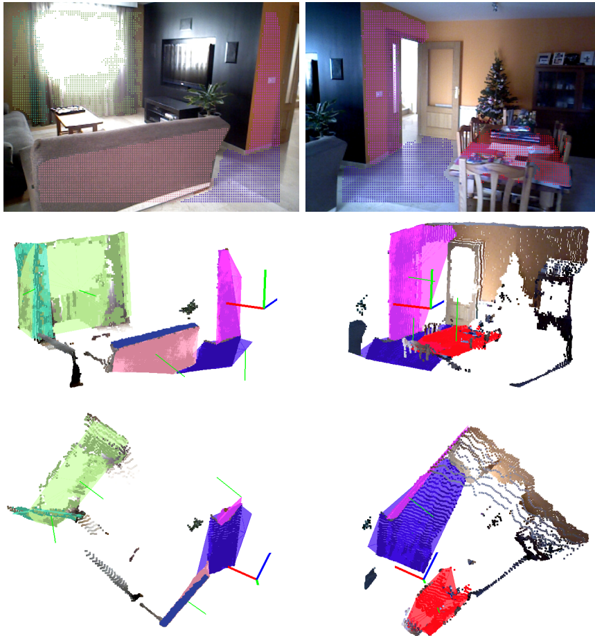
Figure III.8: Corresponding planes in two RGB-D views used to compute their relative transformation. In this example, we use frames 301 and 401 of scene home_at/home_at_scan1_2013_jan_1 from the SUN3D database. Top: plane inliers overlaid on RGB images. Bottom: side and top views showing detected planes in 3D with their normal vectors in thin green and the world frame in red, green and blue lines. Only the blue horizontal and purple vertical planes are common in the two views, but they are sufficient to compute the sensor motion.
