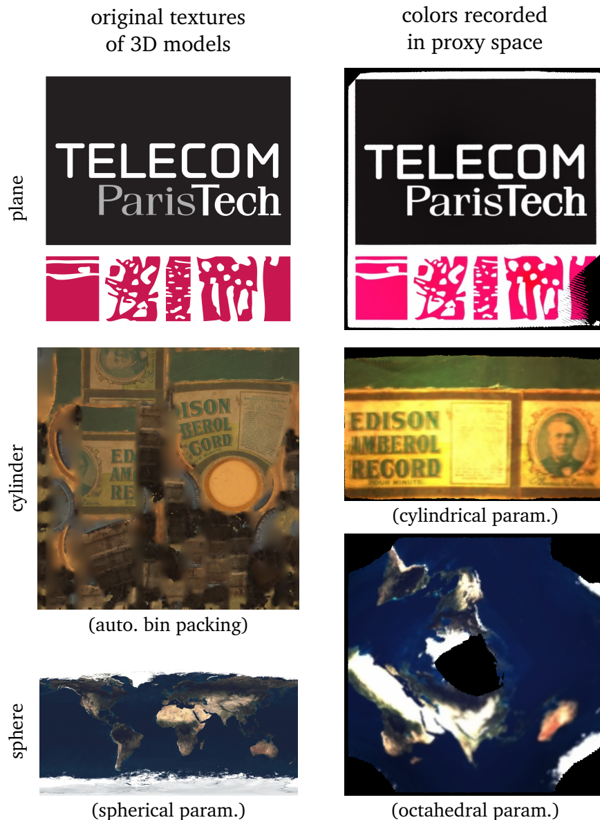
Figure IV.12: Simple shape proxies modeling textures. Left: Texture images from 3D models used to generate the RGB-D sequence in Blender . Right: Our local color point model embedded within the 2D grid of the proxies allows recovering textures of 3D objects. Black areas on the proxies textures were not observed by the camera e.g., the poles of the sphere at the center and corners of the octahedron square (bottom right). As expected, the parameterization of our proxies leads to more consistent and less distorted textures as we can see between e.g., the octahedral and spherical sphere parameterizations (bottom). In addition, our proxies converted the texture of the cylinder from an automatic bin packing to a more meaningful cylindrical parameterized representation (middle).
