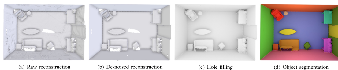
Figure II.13: Planar regularization and segmentation of 3D reconstructions. From the raw scene reconstruction (left), plane regularization and hole filling lead to a more accurate model (middle) which can be easily segmented into planar and non planar connected components (right). Image taken from Dzitsiuk et al. [DSM + 17].
