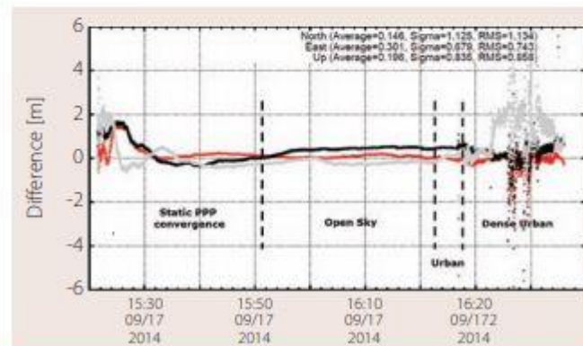
FIGURE 12 Data-authenticated PVT positioning error September 17, 2014, dynamic open sky/urban test
