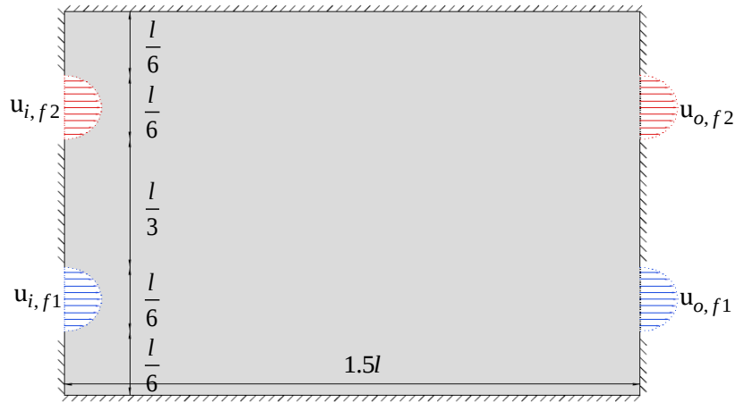
Figure 3.15: Initial configuration of double pipe example with AR=1.5; parallel flow
