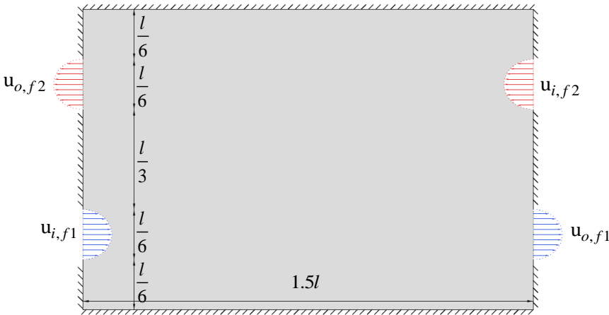
Figure 3.17: Initial configuration of double pipe example with AR=1.5; counter flow
