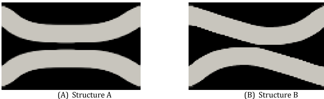
Figure 4.31: Optimal structures for high values of w in parallel flow and counter flow topology optimization
