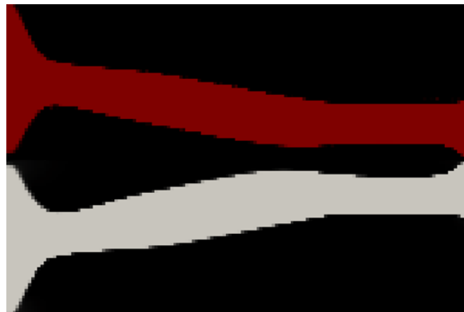
Figure 3.12: Topology optimization result for double diffuser configuration with the modified inverse permeability coefficient
