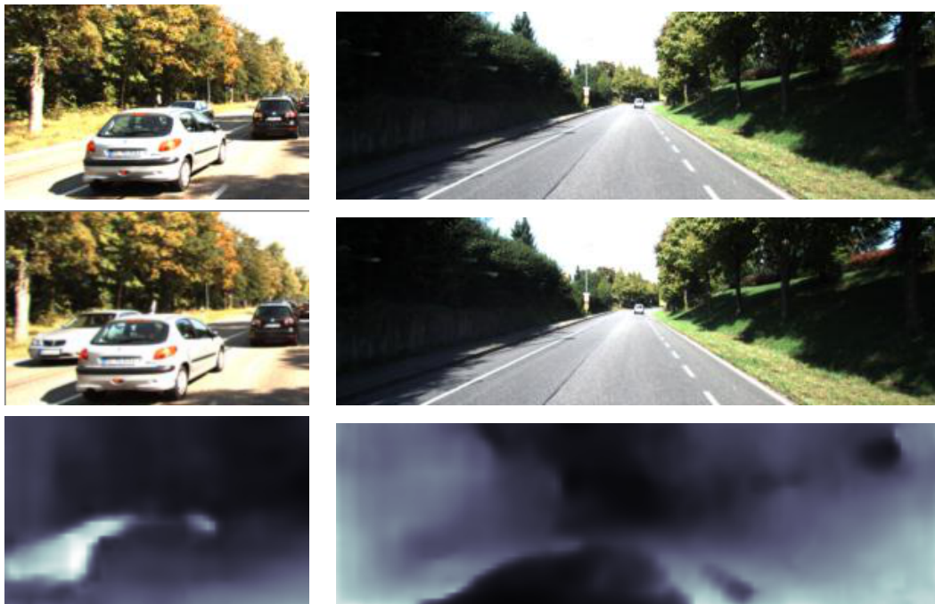
Figure 5.4: Some failure cases of our method on KITTI. First column is a detail of a larger image. The foreground car is moving forward and it's detected as far away, while the background car is moving toward us and is detected as close. Second column is a poorly textured road.
