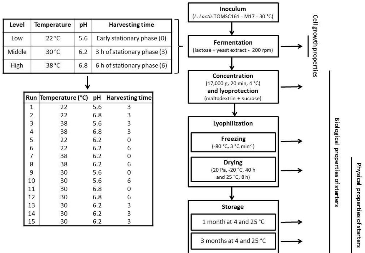
**Figure 1** Diagram of the experimental approach applied for quantifying the effect of fermentation conditions (temperature, pH and harvesting time) on the resistance of *Lactococcus lactis* TOMSC161 to the main steps of the preservation process (freezing, drying and storage)
