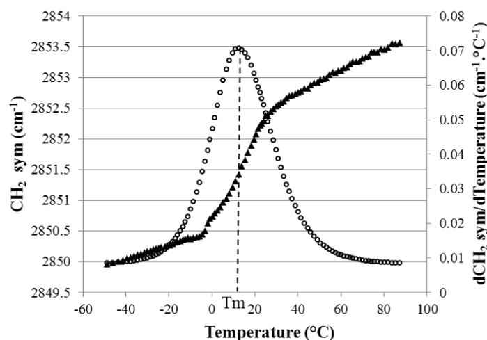
**Fig. 3** Wavenumber of the symmetric CH<sub>2</sub> stretching peak (CH<sub>2</sub>sym) vs. temperature plots (filled triangles), and the corresponding first derivatives (open circles) of *L. lactis* subsp. *lactis* TOMSC161 cells grown at 30 °C and harvested at the early stationary phase (T3).
