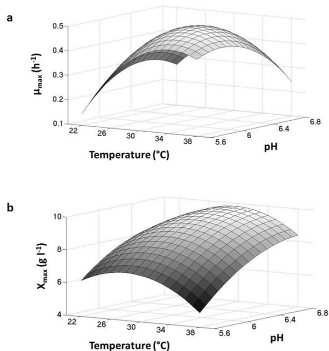
**Figure 2** Response surface representations of the effect of fermentation temperature and pH on the specific growth rate ( $\mu_{\max}$ , in  $\text{h}^{-1}$ ) (a) and on the final biomass concentration ( $X_{\max}$ , in  $\text{g l}^{-1}$ ) (b)
