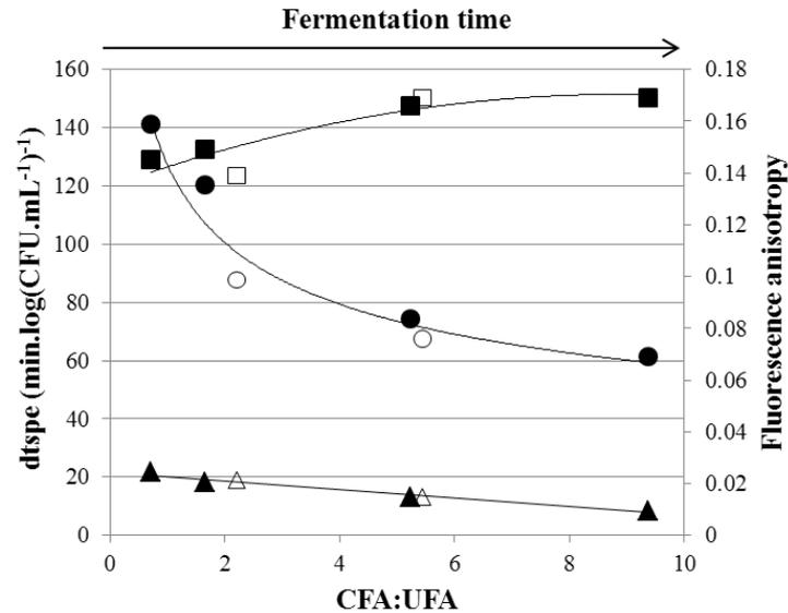
**Fig. 4** Correlation between CFA:UFA ratio, fluorescence anisotropy (squares) and acidification activity loss after freeze-drying (triangles) and after 3 months of storage (circles) of *L. lactis* subsp. *lactis* TOMSC161 grown at different temperatures (22 °C: open and 30 °C: filled) and for the different growth phases studied.
