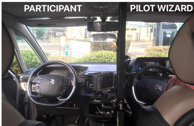
Figure 6.10: The vehicle used for the test drive with the participant’s control interface on the left and the pilot wizard’s controls on the right. The two seats were separated by a panel.
