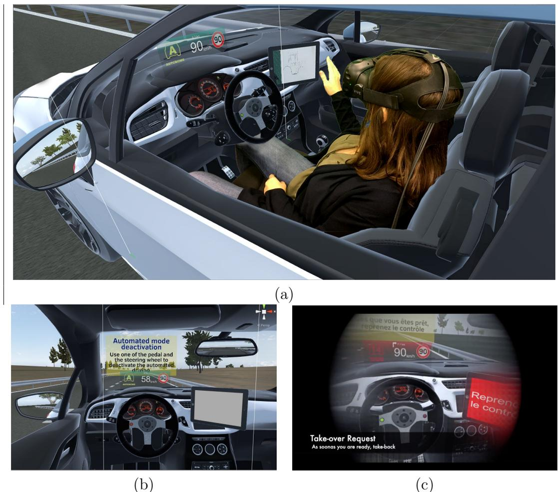
Figure 4.14: The Virtual Learning Environment: (a) a post-production illustration of a participant in the VLE; (b) a view of the interior of the car with the training message (on the transparent panel placed over the steering wheel) and the virtual tablet used for the secondary activity, (c) the reduction of the field of view with the visual tunnel effect
