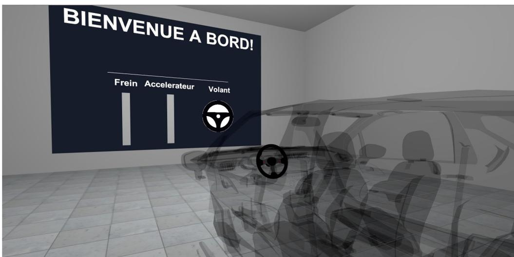
Figure 4.13: The Acclimatization Environment: The car is displayed with a transparent effect and the panel on the front wall shows the indicators for the accelerator and brake pedal and for the steering wheel.
