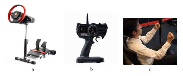
Figure 3.4: Examples of manipulation interfaces for the driving task: (a) a gaming racing wheel and pedals; (b) a RC car remote; (c) a mid-air interaction without hardware [image from F80SAKA [2011]]
