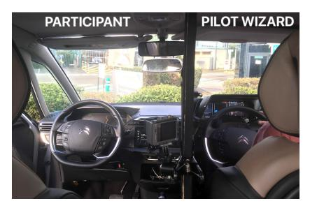
Figure 6.10: The vehicle used for the test drive with the participant's control interface on the left and the pilot wizard's controls n the right. The two seats were separated by a panel.
