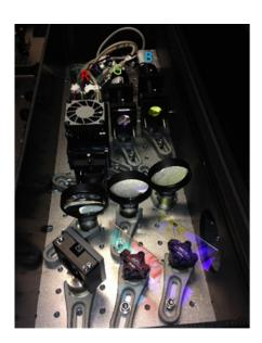
FIGURE 2.8. Detection stage with three independent channels.
