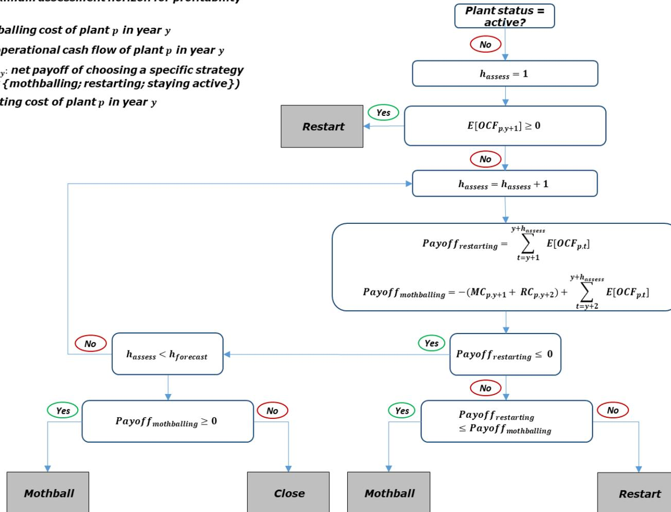
**Figure 69.** Computation of capacity bids for existing plants in capacity markets (when mothballing is not possible)
