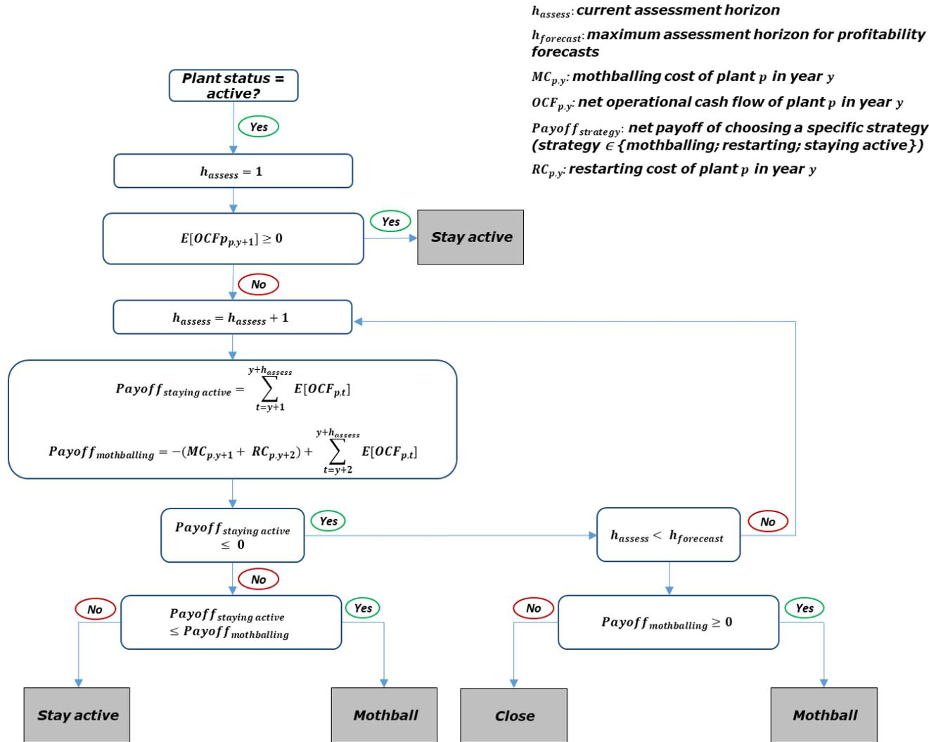
**Figure 68.** Shutdown algorithm for mothballed plants in energy-only markets (when mothballing is possible)
