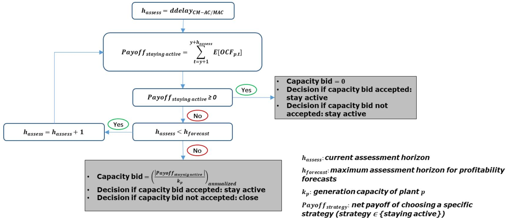
**Figure 70.** Computation of capacity bids for active plants in capacity markets (when mothballing is possible)
