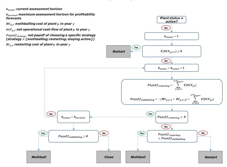
Figure 69. Computation of capacity bids for existing plants in capacity markets (when mothballing is not possible)
