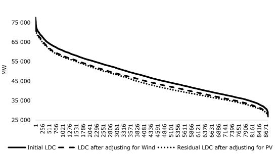
Figure 16. Impact of RES generation on residual load<sup>79</sup>
