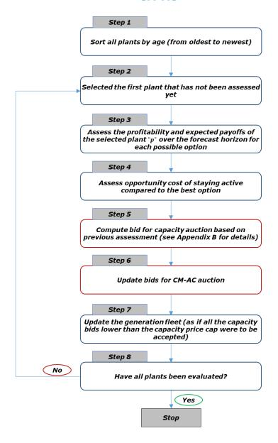
Figure 27. Shutdown/mothballing procedure for existing plants in CM-AC
