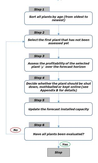
Figure 22. Shutdown/mothballing procedure for existing plants in EOM-PCap/EOM-SP
