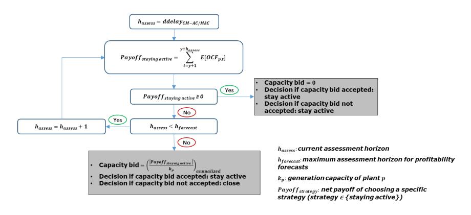
Figure 70. Computation of capacity bids for active plants in capacity markets (when mothballing is possible)
