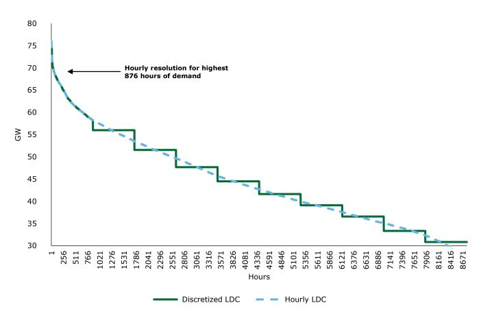
Figure 74. Discretization of LDC in forecasts in Chapters II and III
