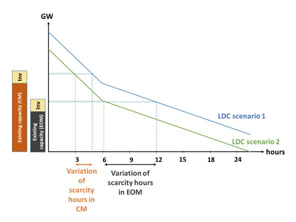
While assessing the profitability of a new generation unit, investors usually resort to expected demand curves and compute estimated revenues. Conceptually, this process can be represented by using load duration curves (LDCs), which correspond to hourly load levels sorted in decreasing order. By construction, the
