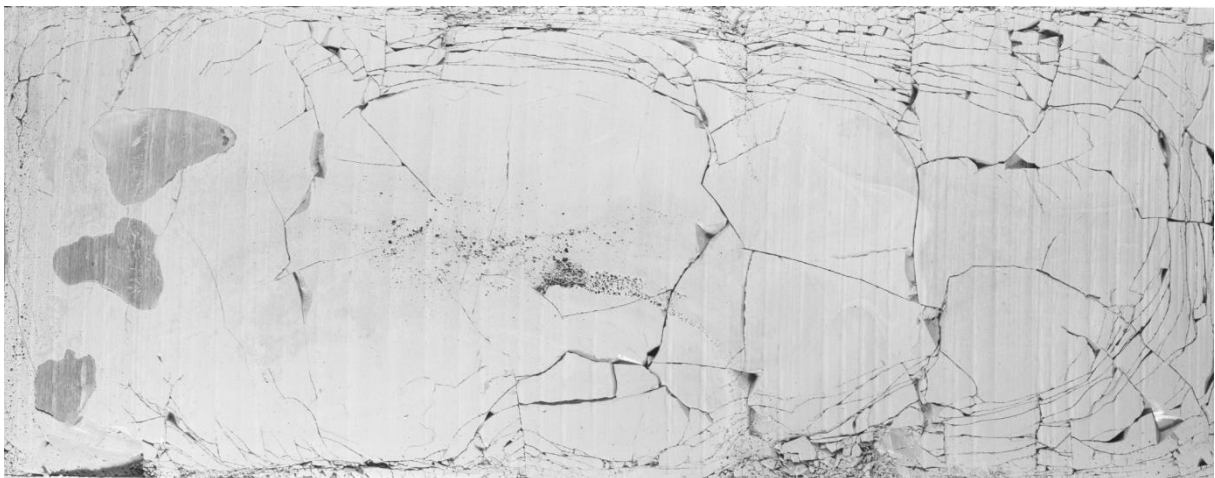
Figure 3-5 Grayscale image of the UMo block of vitrified fractured glass. Dimensions: 1044 mm × 413 mm.
