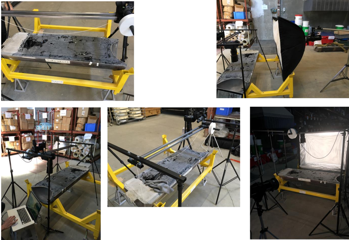
Figure 3-9 Working process undertaken to realize a series of high-quality ordinary images of fracture network of two inactive vitrified nuclear glass canisters.
