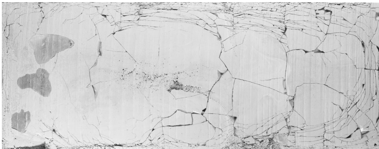
Figure 2 Grayscale image of the UMo bloc of vitrified fractured glass. Dimensions: 1044 mm × 413 mm.
