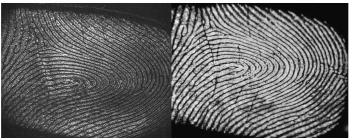
Figure 4.6 – Comparison of internal fingerprints taken by FFOCT with external fingerprints taken by FTIR [185]. (left) In vivo FFOCT image of internal fingerprint taken a few hundred micrometers below the skin surface and (right) total reflection image of the same external fingerprint (inversed contrast).
