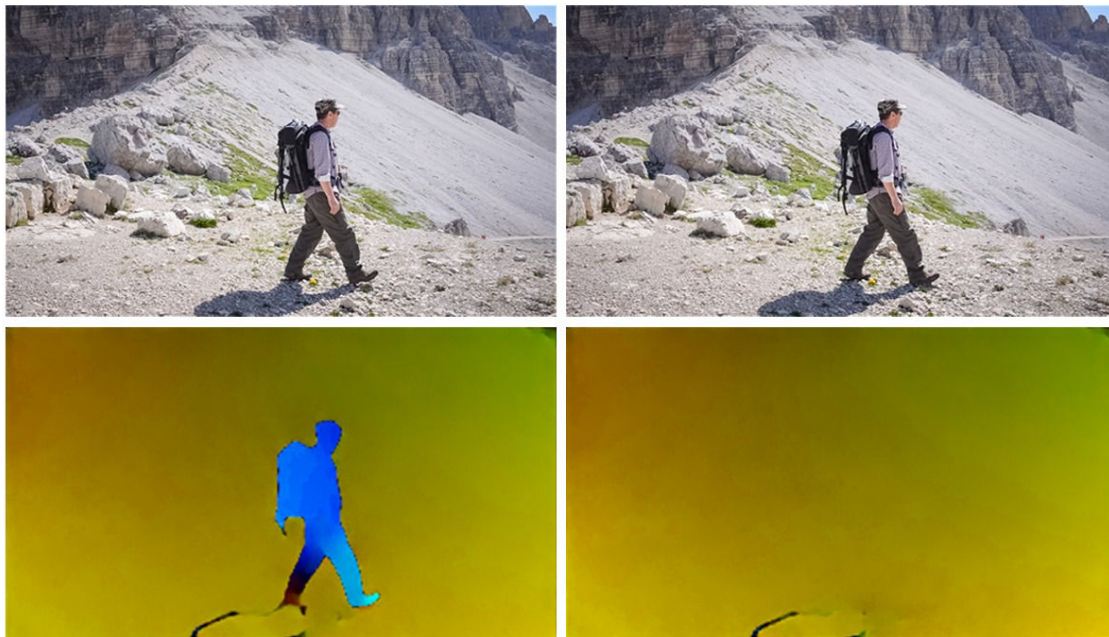
Figure 4.7 – Motion field reconstruction by inpainting the optical flow field. From two consecutive images (top row), we compute the optical flow field by FlowNetv2 (bottom left), then we use an image inpainting method to reconstruct the optical flow field inside the occlusion (bottom right).
