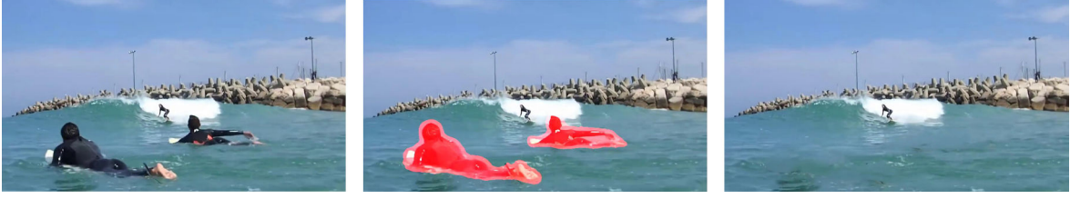
Figure 2.17 – The inpainting problem. Left: original image; middle: inpainting mask \mathcal{H} , in red; right: an inpainting result.
