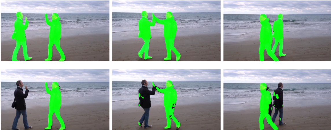
Figure 3.18 – OSVOS method can distinguish well between background and foreground, but it has difficulties when separating similar instance of the same semantic class. Top: Results when we want to segment both persons. Bottom: results when we only want to segment the person on the right.
