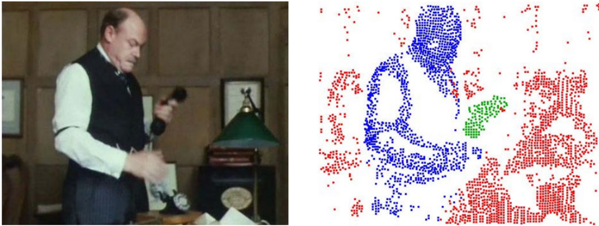
Figure 3.5 – Unsupervised video segmentation based on point trajectories clustering. Left: A sample frame input. Right: Long term motion analysis is used to separate the man, telephone receiver from the background. Image from (Brox and Malik 2010)
