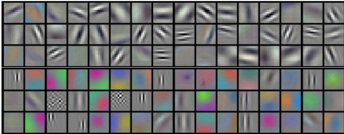
Figure 2.4 – Visualization of example filters learned by AlexNet (Krizhevsky, Sutskever, and Hinton 2012). Source O'Reilly's library.
