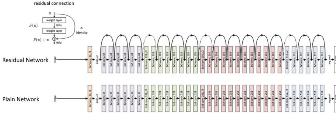
Figure 2.6 – Residual Network architecture with residual connection (top row). Plain network architecture without residual connection (bottom row). Image taken from (He, X. Zhang, et al. 2016).
