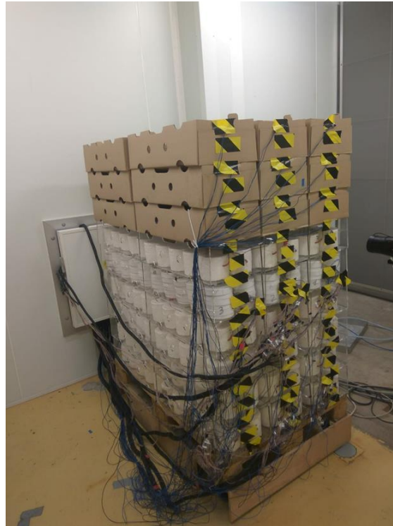
Figure V-12 Obstructed lateral vent holes
