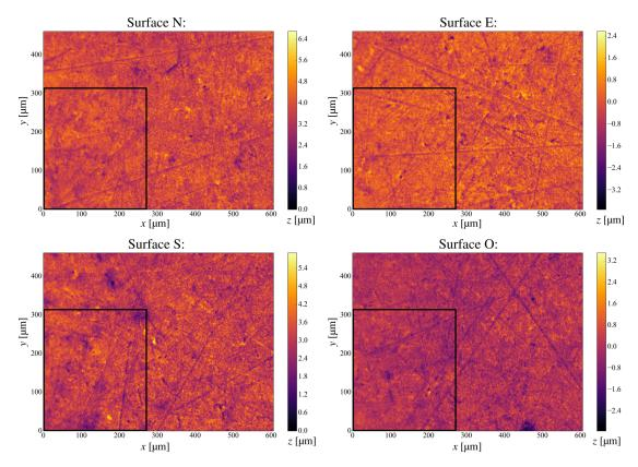
Figure 9.11: Surface topography measurements of 4 zones of the Stellite seal ( $736 \times 480$  measurement points). Black frame shows the part of the surface used in simulations ( $325 \times 325$  points).
