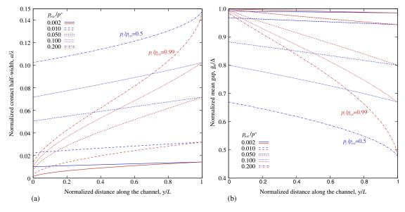
Figure 8.4: Approximate solutions for (a) normalized contact region half-width  $a/\lambda$  and (b) normalized mean gap  $\bar{g}_n/\Delta$  evolution along the channel.
