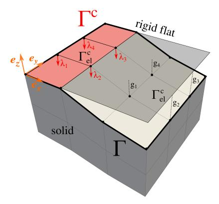
Figure 4.4: Sketch of the interface highlighting contact elements:  $\Gamma$  is the potential contact zone,  $\Gamma^c$  is the active contact zone (active set),  $\Gamma^c_{\rm el}$  is a face associated to one contact element,  $\lambda$  is the Lagrange multiplier, which represents contact pressure and is attributed to each node of the surface  $\Gamma$ ,  $g_n$  is the gap function:  $g_n = 0$  on  $\Gamma^c$  and  $g_n > 0$  on  $\Gamma \setminus \Gamma^c$ .
