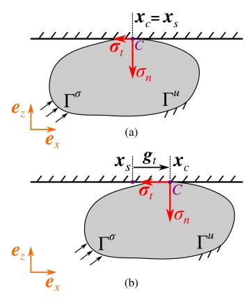
Figure 2.4: Unilateral frictional contact: (a) material point C is in the *stick* state, and  $\boldsymbol{x}_s$  is the position it adheres to; (b) point C is in the *slip* state, and  $\boldsymbol{g}_t$  is the tangential slip with respect to the stick position  $\boldsymbol{x}_s$ .
