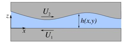
Figure 2.8: Fluid flow in a thin channel between two solids: one of the two surfaces is flat and aligned with the plane z = 0, while the other surface is given by an equation z = h(x, y), where h determines the film thickness.
