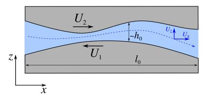
Figure 2.7: Fluid flow in a thin channel between two solids:  $h_0$  is the characteristic thickness of the fluid film, and  $l_0$  is the scale of the lateral extent of the channel in the x-direction. Note that the scales corresponding to the y-direction are not shown to avoid overcrowding.
