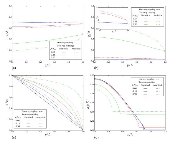
Figure 8.8: Comparison of results of numerical simulations with the approximate analytical solutions for (a) normalized contact region half-width  $a/\lambda$ , (b) normalized mean gap  $\bar{g}_n/\Delta$  and (c) normalized fluid pressure  $p/p_i$  evolution along the channel, (d) normal traction component  $|\sigma_n|/E^*$  in the section y = L/2.
