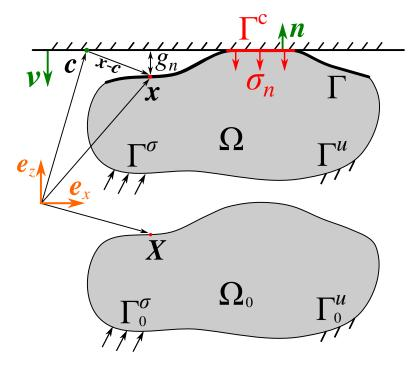
Figure 2.3: Unilateral contact between a deformable solid and a rigid flat:  $\Gamma$  is the *potential* contact zone, and  $\Gamma^{c} \subset \Gamma$  is the *active* contact zone.
