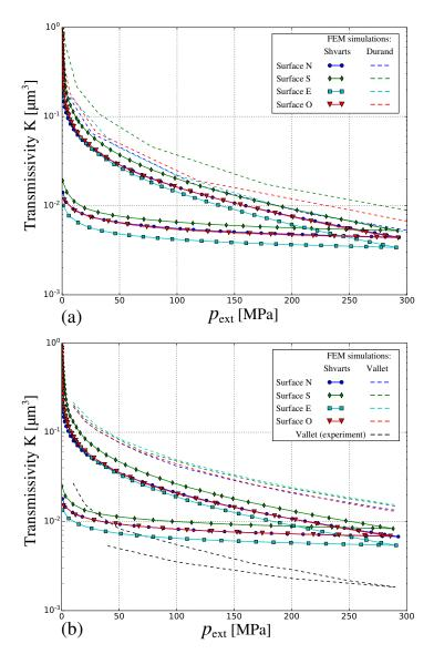
Figure 9.13: Evolution of the interface transmissivity during loading-unloading process. Simulations performed using material properties of two alloys: (a) Norem and (b) Stellite.
