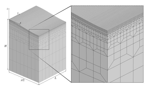
Figure 8.5: Finite element mesh with  $128 \times 128$  elements on the contact surface, which was used to solve the coupled solid-fluid problem.
