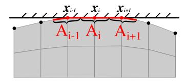
Figure 4.2: Definition of the area  $A_i$  corresponding to *i*-th contact element in the node-to-rigid-surface discretization approach.
