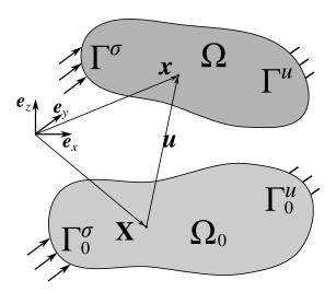
Figure 2.1: Reference (initial) configuration  $X \in \Omega_0$  and current (deformed) configuration  $x \in \Omega$  of the deformable solid; u = x - X is the displacement vector field.
