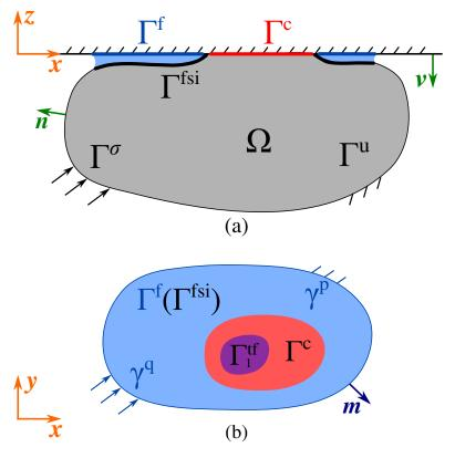
Figure 2.11: Sketch of the problem under study: (a) contact between a solid and a rigid plane with fluid present in the interface; (b) view of the contact interface. Notations:  $\Gamma^c$  is the active contact zone,  $\Gamma^f$  is the lubrication surface (where the Reynolds equation is solved),  $\Gamma^{fsi}$  is the fluid-structure interface,  $\Gamma^{ff}_1$  is a trapped fluid zone, see (2.67). Note that  $\Gamma^f$  is the projection of  $\Gamma^{fsi}$  on the rigid flat.
