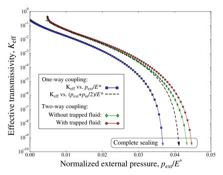
Figure 8.13: The evolution of the effective interface transmissivity  $K_{\rm eff}$  under increasing external load with comparison between 3 simulations: one-way coupling approximation, two-way coupling neglecting effect of the trapped fluid and two-way coupling with the trapped fluid. Additionally, the results of the one-way coupling simulation are shown shifted by an offset of the external load equal to  $p_{\rm in}/2$  (see explanations in the text).
