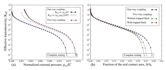
Figure 9.3: Fluid flow through representative rough contact interface: comparison of the effective transmissivity for different coupling approaches.
