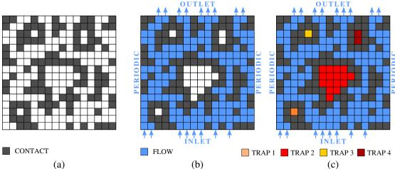
Figure 6.3: Identification of active contact (a), fluid-flow (b) and trapped fluid zones (c) by performing the connected-component labelling of the interface graph based on the 4-connected neighbourhood: two faces are connected if they share an edge.
