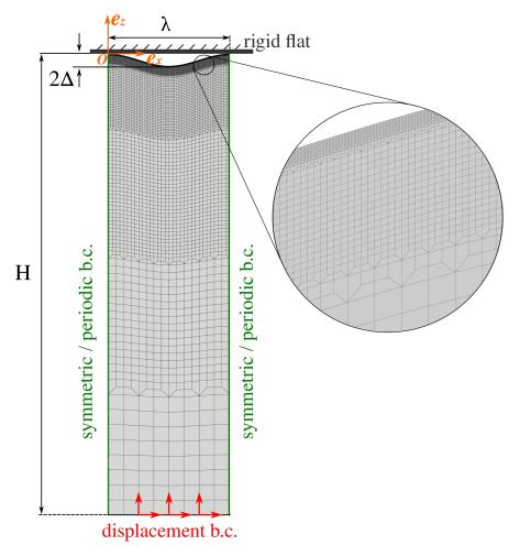
Figure 7.2: Finite-element mesh and boundary conditions for the trapped fluid problem. Several loading scenarios are considered, corresponding to *frictionless* and *frictional* simulations. Accordingly, on the vertical walls  $x = 0, x = \lambda$  either symmetric or periodic boundary conditions are enforced, and on the bottom edge of the solid z = -H either only vertical displacement, or a vertical displacement followed by a horizontal one is applied.
