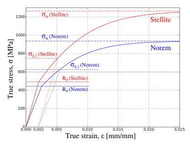
Figure 9.10: Stress-strain curves of two studied alloys, corresponding to the non-linear hardening model (9.12).
