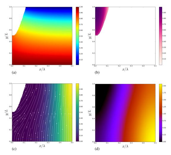
Figure 8.6: Results of the numerical simulation: (a) normalized fluid pressure  $p/p_i$ , (b) normalized contact pressure  $|\sigma_n|/|\sigma_n|^{max}$ , (c) normalized fluid flux intensity  $|q|/|q_{max}|$ , (d) normalized gap  $g/\Delta$ ;  $p_{\rm ext}/p_W^* = 0.48$ ,  $p_i/p_W^* = 0.72$ , which corresponds to  $p_i/p_{\rm ext} = 1.5$ .
