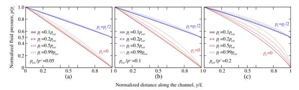
Figure 8.3: Approximate solution (8.16) for the mean hydrostatic fluid pressure distribution along the wavy channel in contact with a rigid flat for  $p_o = p_i/2$  and  $p_o = 0$  (a)  $p_{\rm ext}/p_W^* = 0.05$ , (b)  $p_{\rm ext}/p_W^* = 0.1$ , (c)  $p_{\rm ext}/p_W^* = 0.2$ ; the fluid pressure is normalized by the inlet pressure  $p/p_i$  and the coordinate is normalized by the channel length y/L.
