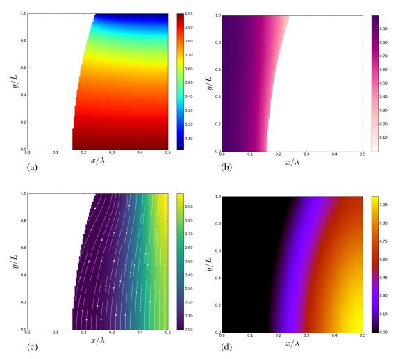
Figure 8.7: Results of the numerical simulation: (a) normalized fluid pressure  $p/p_i$ , (b) normalized contact pressure  $|\sigma_n|/|\sigma_n|^{max}$ , (c) normalized fluid flux intensity  $|q|/|q_{max}|$ , (d) normalized gap  $g/\Delta$ ;  $p_{\rm ext}/p_W^*=0.8$ ,  $p_i/p_W^*=0.72$ , which corresponds to  $p_i/p_{\rm ext}=0.9$ .
