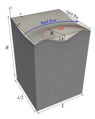
Figure 8.11: Finite-element mesh with  $128 \times 128$  faces in the contact interface which was used to solve the problem of the fluid flow across a channel with an "atoll" island. Note that the amplitude of the surface profile is exaggerated to highlight its features, while in the actual simulation the following geometrical parameters were used:  $\Delta = 0.02 \text{ mm}, \lambda = 2 \text{ mm}, L = 1 \text{ mm}, B = 1.4 \text{ mm}, R_a = 0.333 \text{ mm}, \alpha = 9 \text{ mm}^{-2}$ .
