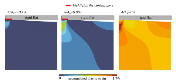
Figure 7.9: Accumulated plastic strain near the contact interface is shown at three different external loads for the incompressible fluid and for  $V^{\rm tf}/V_0 = 0.9$  and  $\Delta/\lambda = 0.01$ , from left to right: (1) the step corresponding to activation of the fluid; (2) the plastic zone appears in the valley between the asperities; (3) opening of the trap (contact area is zero; as seen from the plastic field, at this moment the entire solid is plastified).
