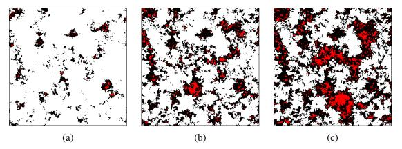
Figure 1.1: Morphology of the contact interface between an elastic half-space with a rough surface and a rigid flat under increasing external load, numerical simulation results [Yastrebov et al., 2015]: black is the real contact area, white is the "free" out-of-contact area and red is the "trapped" out-of-contact area, bounded inside non-simply connected contact patches.
