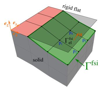
Figure 6.2: Sketch of the interface highlighting FSI elements:  $\Gamma^{\text{fsi}}$  is fluid-structure interface on the surface of the solid,  $\Gamma^{\text{fsi}}_{\text{el}}$  is a face associated to one FSI element, p is the fluid pressure at each node of this surface and n is the outer normal.
