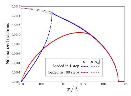
Figure 7.11: Comparison of two frictional (normal loading only) contact simulation with the same final normal load ( $p_{\text{ext}}/E^* = 0.00018$ ), but different loading sequences: the full load is applied in either 1 or 100 load steps. Full curves with markers represent frictional (shear) traction, while dashed ones show normal traction multiplied by the CoF  $\mu = 0.3$ . Both tractions are normalized by  $E^*$ .
