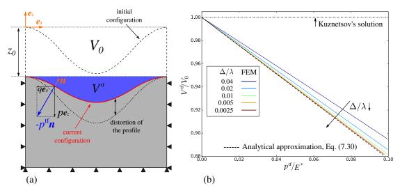
Figure 7.4: (a) Sketch of the auxiliary problem: deformation of the wavy surface under uniform hydrostatic pressure. (b) Evolution of the ratio  $V^{\rm tf}/V_0$  ( $V^{\rm tf}$  is the volume between the deformed surface and a horizontal plane  $z=z_0$ , where  $z_0$  is the current position of the crest, and  $V_0$  is the initial volume of the gap) with the increasing hydrostatic pressure  $p^{\rm tf}$  for several profiles with different slope  $\Delta/\lambda$ .
