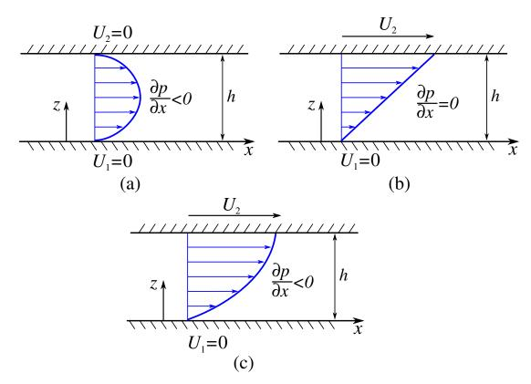
Figure 2.9: Velocity profiles for: (a) Poiseuille pressure-driven flow between immobile walls; (b) Couette shear-driven flow due to the relative motion of the walls; (c) Combination of the Poiseuille and the Couette flow.
