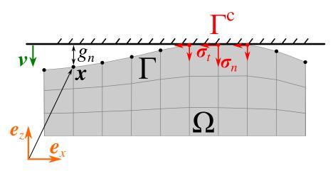
Figure 4.1: Node-to-rigid-surface contact discretization:  $\Gamma$  is the potential contact zone,  $\Gamma^c$  is the active contact zone.
