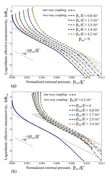
Figure 9.6: Fluid flow through representative rough contact interface: comparison of the effective transmissivity: for (a) fixed outlet pressure and several inlet pressures, (b) fixed inlet pressure and several outlet pressures.
