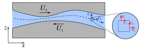
Figure 2.5: Laminar fluid flow between two surface with macroscopic velocities  $U_1$  and  $U_2$ . Note that the fluid velocity and stress components corresponding to the y-direction are not shown to avoid overcrowding.
