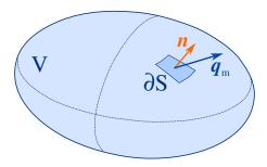
Figure 2.6: Outflow of fluid from a volume V, bounded by a surface S: n is the outer normal to a surface element  $\partial S$  and  $\boldsymbol{q}_m$  is the mass flux vector.
