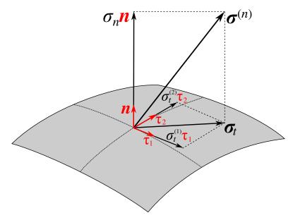
Figure 2.2: Normal  $\sigma_n \mathbf{n}$  and tangential  $\sigma_t$  components of the traction vector  $\boldsymbol{\sigma}^{(n)}$ , corresponding to a normal  $\boldsymbol{n}$ .
