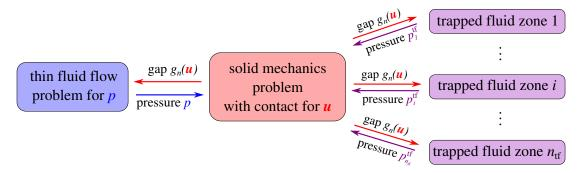
Figure 2.12: Schematic diagram showing dependencies between coupled sub-problems.
