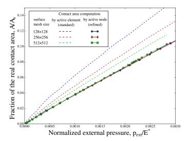
Figure 9.8: Comparison of two different methods of the real contact area computation: (4.120) and (4.121). Results of simulations using three different meshes are presented (with  $128 \times 128$ ,  $256 \times 256$  and  $512 \times 512$  face elements on the surface).
