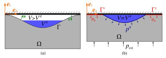
Figure 5.1: (a) Trapped fluid is in inactive state. (b) Trapped fluid is in active state. Note that the presented sketch corresponds to the plane strain problem statement (no dependency on the y-coordinate): fluid is trapped inside of a "valley" contained between two contact zones. In a 3D problem set-up fluid entrapment is possible only inside of a "pool" bounded by a non-simply connected contact patch.
