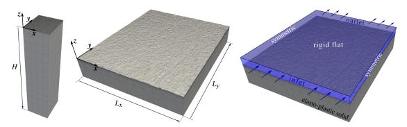
Figure 9.9: A sketch of the problem set-up: contact between a deformable solid with a rough surface and a rigid flat in presence of the thin fluid flow in the free volume between two surfaces.
