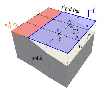
Figure 6.1: Sketch of the interface highlighting fluid flow elements:  $\Gamma^{\rm f}$  is the lubrication surface (plane z=0), where the Reynolds equation is defined,  $\Gamma^{\rm f}_{\rm el}$  is a face on this surface associated to one fluid flow element, p is the fluid pressure DOF, added to each node of the surface of the solid (note that the constant fluid pressure across film thickness is assumed).
