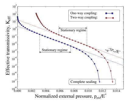
Figure 9.5: The decrease of the transmissivity with the increasing external load, shown for one- and two-way coupling simulations. The stationary regime corresponding to the exponential decay is highlighted.
