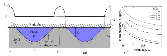
Figure 8.2: (a) - Contact between an elastic wavy profile and a rigid flat with a pressurized fluid in the interface, (b) - variation of the mean pressure on the surface with the mean gap.
