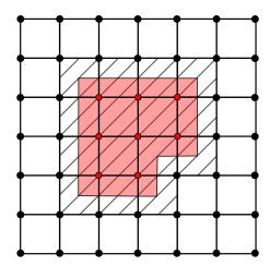
Figure 4.5: Sketch on the computation of the real contact area. Red circles represent nodes with  $\hat{\lambda}_i \leq 0$ , black ones correspond to  $\hat{\lambda}_i > 0$ . The dashed area represents the contact area computed by summing up areas of all active elements, see (4.120). The shaded area is obtained by a refined approach of summing up areas corresponding to nodes with  $\hat{\lambda}_i \leq 0$ , computed using the nearest Gauss point to node i, see (4.121).
