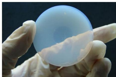
Figure 17. Example of silica aerogel monolith (from TEOS) presenting a density of 0.13 g cm -3 and an effective thermal conductivity of 0.015 W/(m.K.). Reprinted by permission from [Springer Nature] [Journal of Sol-Gel Science and Technology] [from (M. Koebel et al., 2012)], [COPYRIGHT] (2019).
