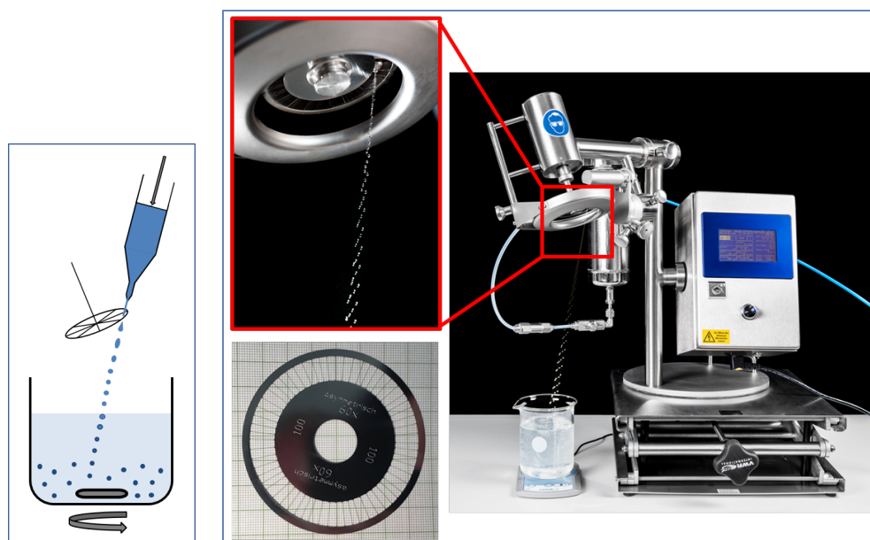
Figure 2.8 – Schematic representation (left) and pictures of the JetCutter (right) and one of the cutting tools used (bottom middle). Pictures provided by GeniaLab (Germany).
