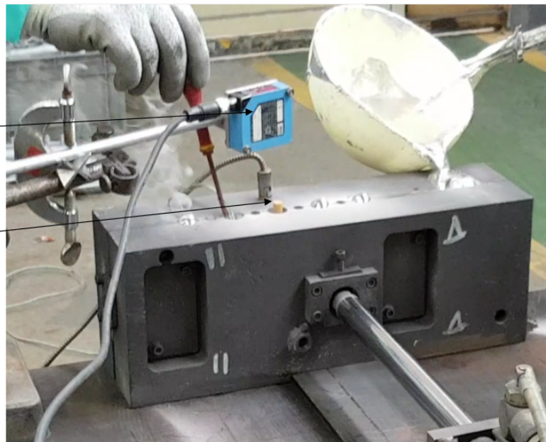
Figure 5.18: Technological specimen "CDG" instrumented with a laser sensor during casting
