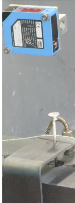
Figure 5.17: Ceramic rod insertion and laser sensor set up
