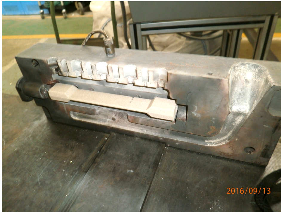
Figure 5.5: View of the “dog bone” specimen placed inside the “clarinet” mold
