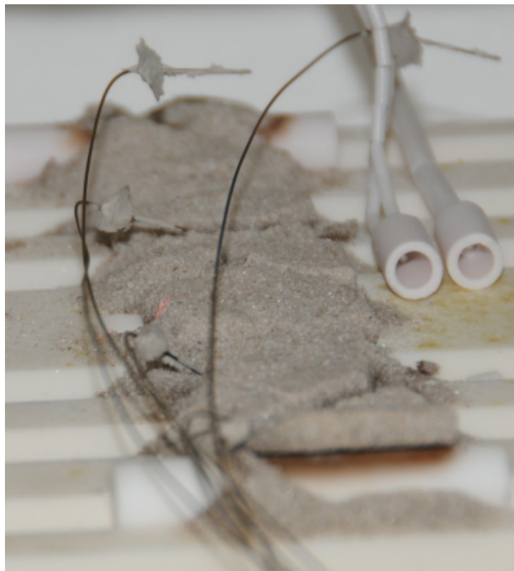
Figure 3.18: Sand core specimen heated up to 450 °C during the instrumentation.
