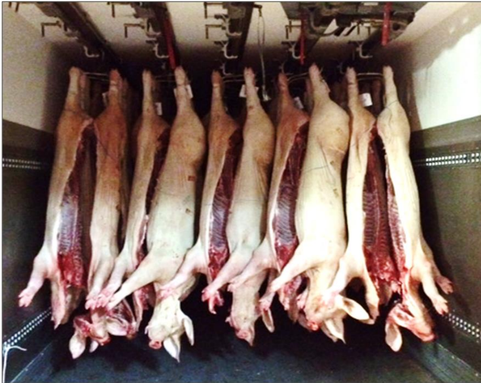
Figure 2-1 : Photo of a refrigerated trailer with 5 rails loaded with pork carcasses as the studied configuration.
