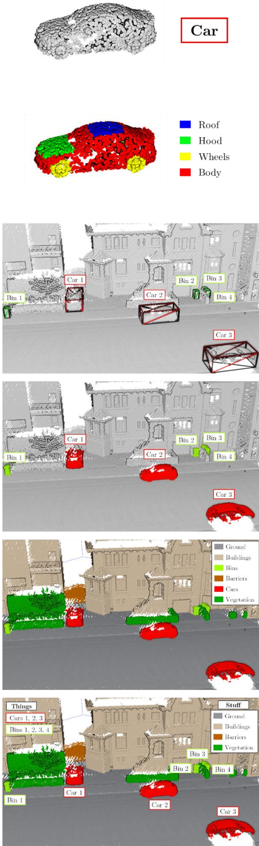
Figure 2. Illustration of the hierarchy of semantic understanding tasks on point clouds.
