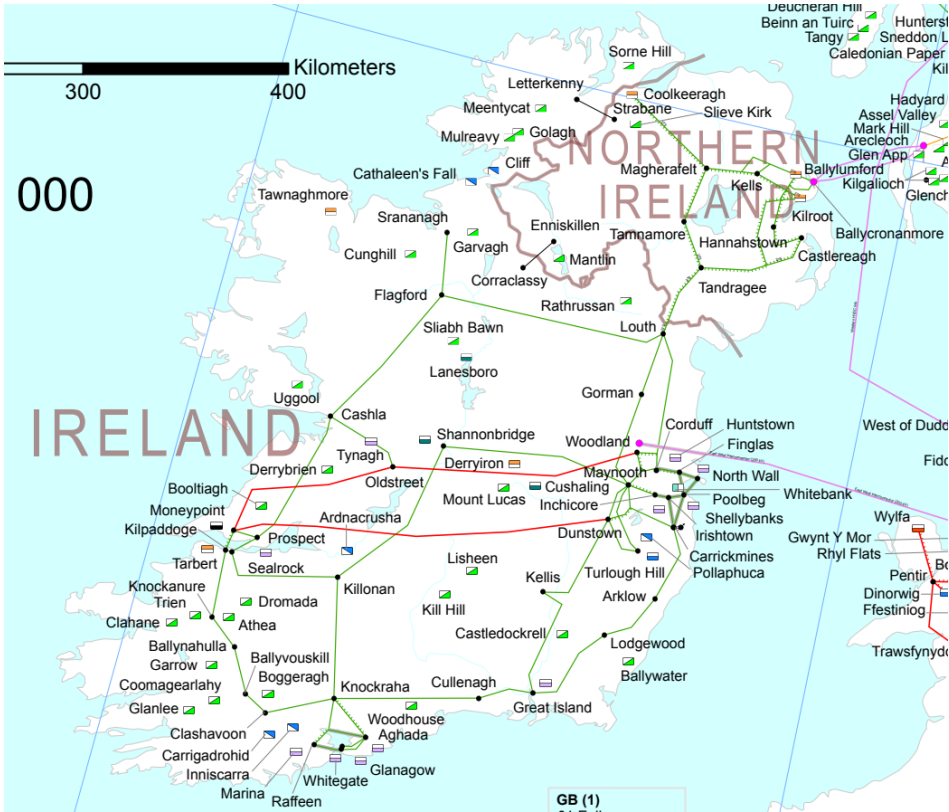
Figure 4.10: Structure of the Irish transmission system
