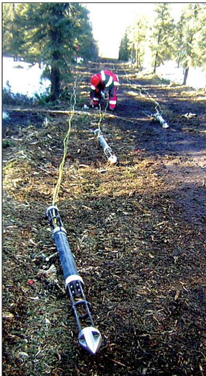
**Figure 1.** SeisMovie sources laid out prior to installation. The piezoelectric stack is mounted in a “cage” about 2 m long and cemented into the borehole at a depth of 80 m.
