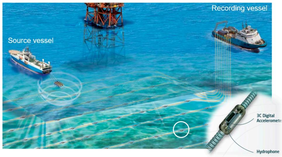
Figure 12: Ocean Bottom Cable seismic operation with the Sercel SeaRay 428. The SeaRay encompasses three orthogonally oriented, digital accelerometers and a hydrophone to form a single four component (4C) receiver. Courtesy of Sercel.
