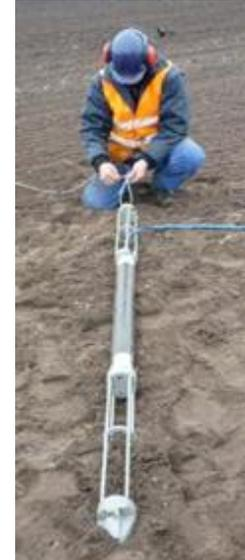
Figure 4: A SeisMovie™ piezoelectric source ready to be cemented in the downhole.
