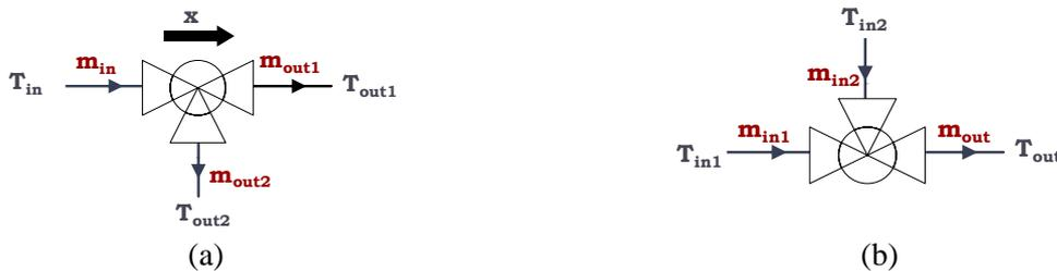
Figure 3.25. (a) Splitter unit, (b) mixer unit
