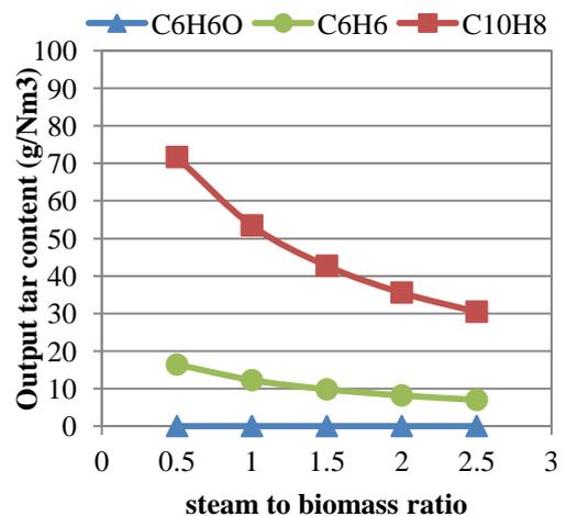
Figure 3.12. Steam to biomass effect on the tar content of the gasifier's output
