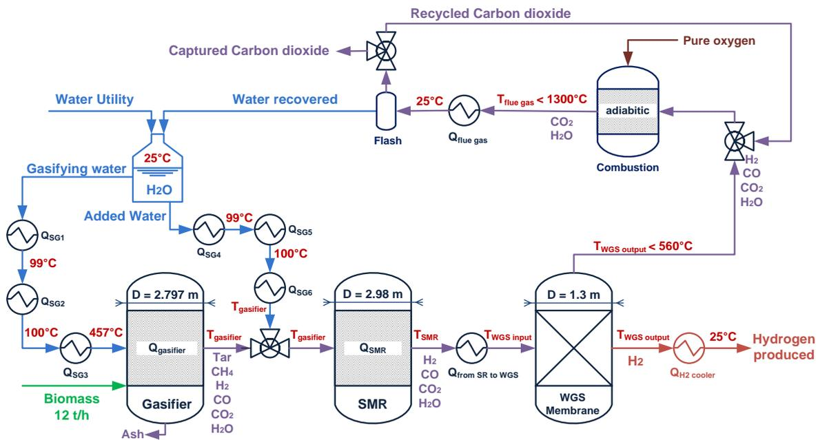
Figure 4.5. Wood to hydrogen conversion process flow sheet
