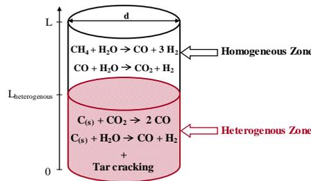
Figure 3.8: The chemical reactions taking place in the gasifier
