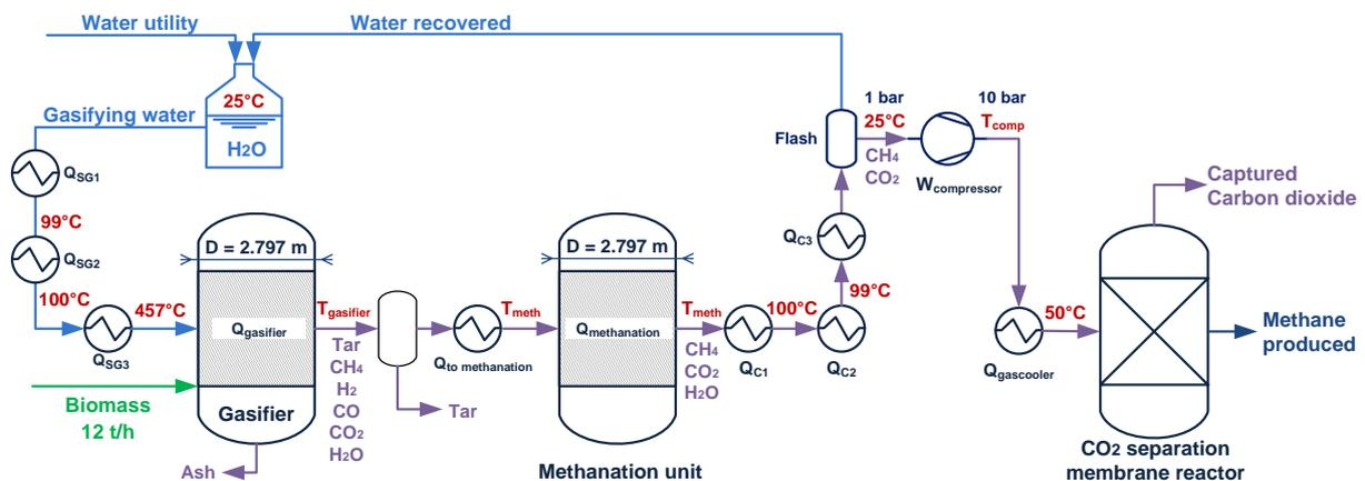
Figure 4.6. Wood to methane conversion process flow sheet
