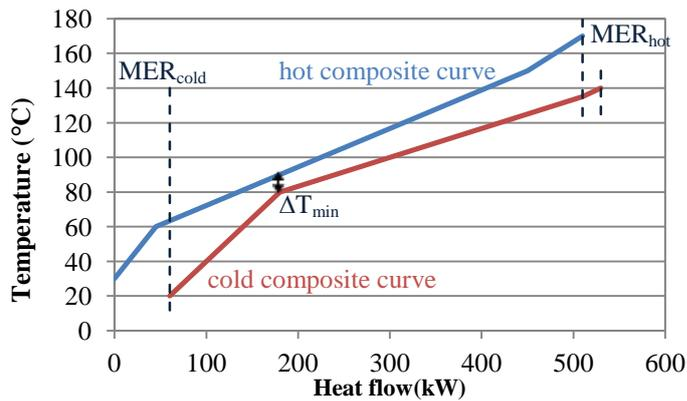
Figure 1.9. Hot and cold composite curves representation
