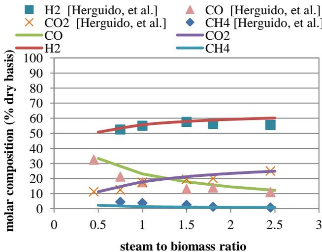
Figure 3.11. Steam to biomass effect on gas composition
