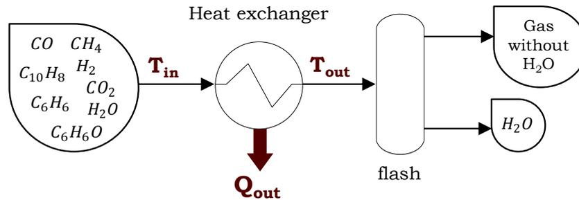
Figure 3.17. Water separation unit
