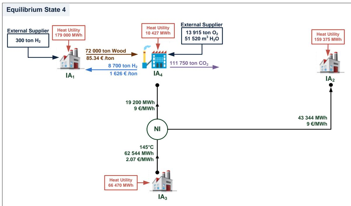
Figure 4.40. EIP configuration of the most adequate equilibrium state in non-cooperative scheme
