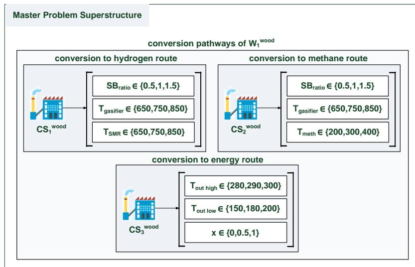
Figure 4.8. Superstructure of W<sub>1</sub><sup>wood</sup> conversion pathways
