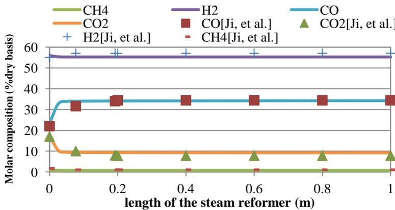
Figure 3.14. Gas composition profile along the steam reformer
