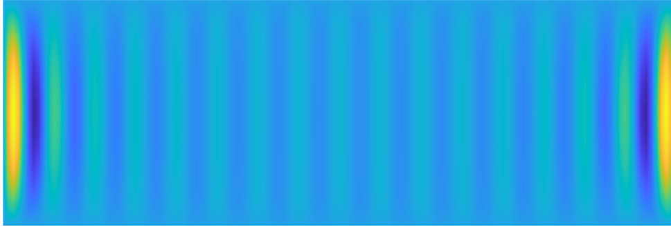
Figure 4.4 Imperfection of the membrane for wrinkling, tension load 0.02mm, imperfection 0.001mm.
