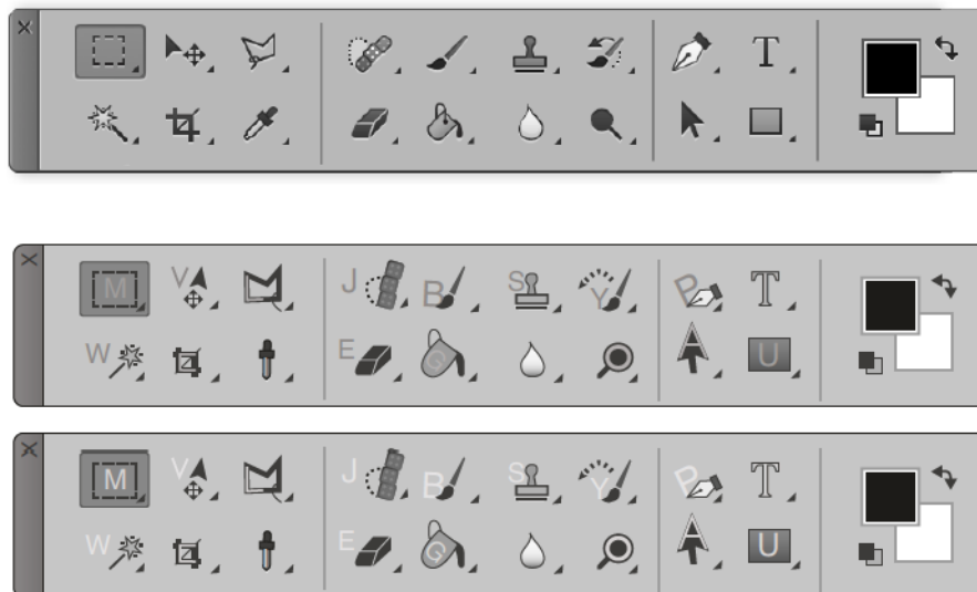
Figure 4.12: Possible adaption of the Adobe Photoshop CC 2015 interface using IconHK. Top: default toolbar. Middle & Bottom: the adapted toolbar integrating IconHK principles at two different levels of magnification. All buttons embed their associated hotkey, except the Blur button (water drop) which lacks a hotkey.
