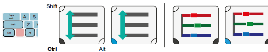
Figure 4.7: Example of icons augmented with iconHK that embed modifiers using the keyboard-location inspired mapping: alt at the bottom-right, Ctrl at the bottom-left, shift at the top-left. The commands equal line space (left) and RGB colors (right) respectively have Ctrl + E and Ctrl + alt + E as keyboard shortcuts. Corners are filled in dark to convey modifiers involved in the shortcuts (bottom-left corner only for equal line space , two bottom corners for RGB colors ). The bottom-left corner is highlighted in blue when Ctrl is pressed to provide feedback.
