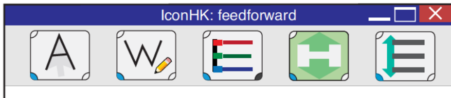
Figure 4.10: When the user presses a modifier key, the magnification factor of all buttons increases to M_{\square} to maximize the saliency of the hotkey when the user needs them the most.
