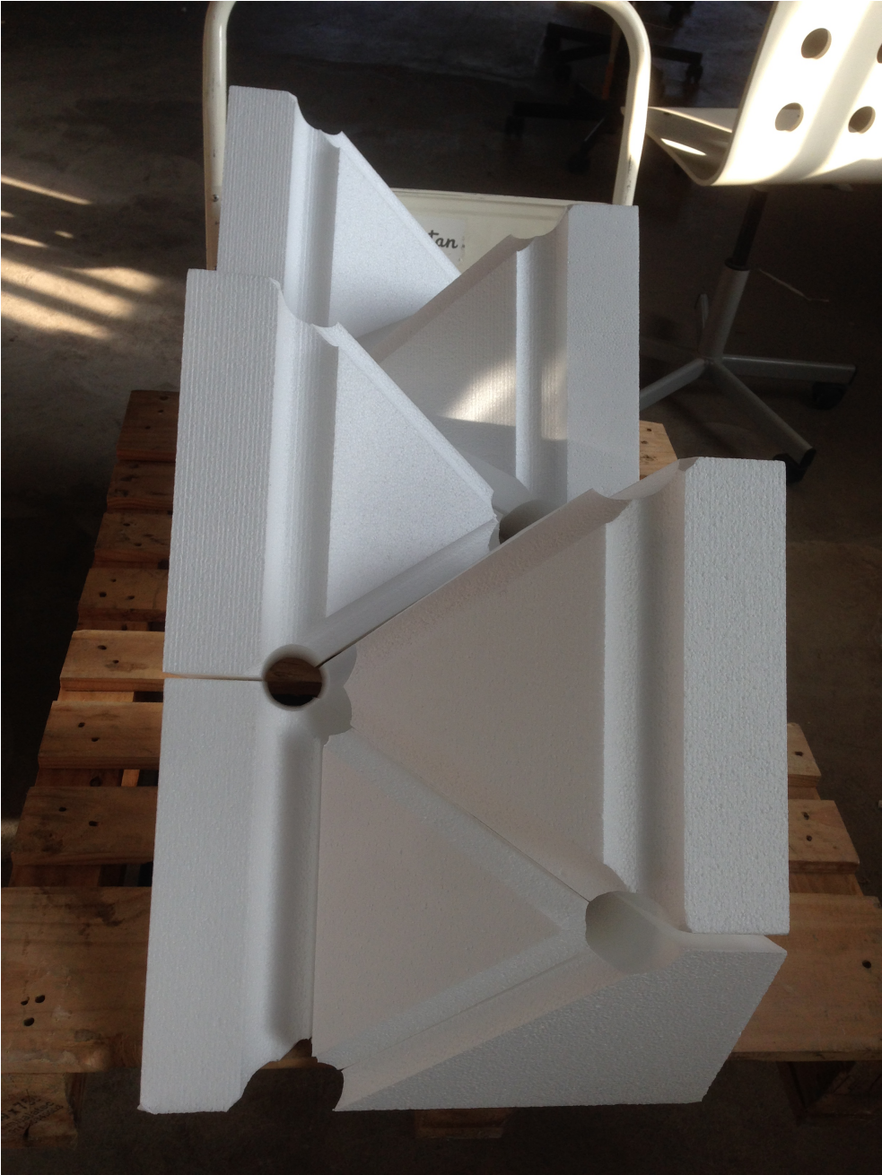
Figure 5.12: EPS blocks forming channels
