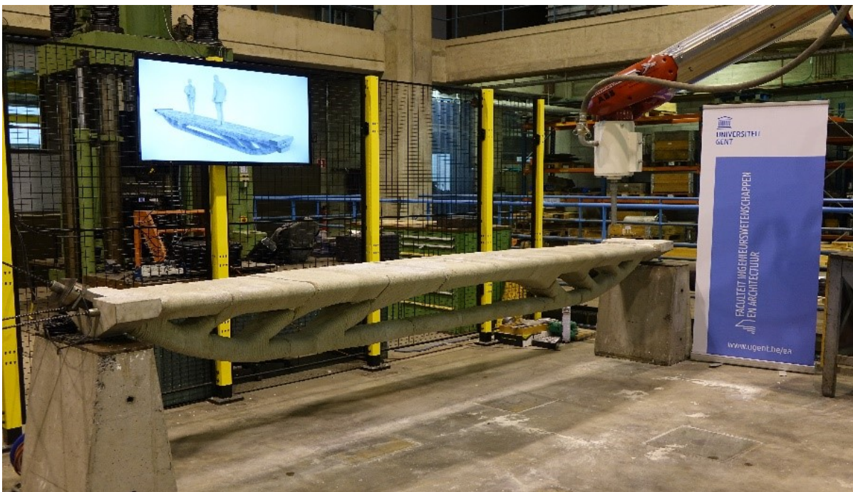
Figure 6.5: An "optimal concrete bridge" from Ghent university
