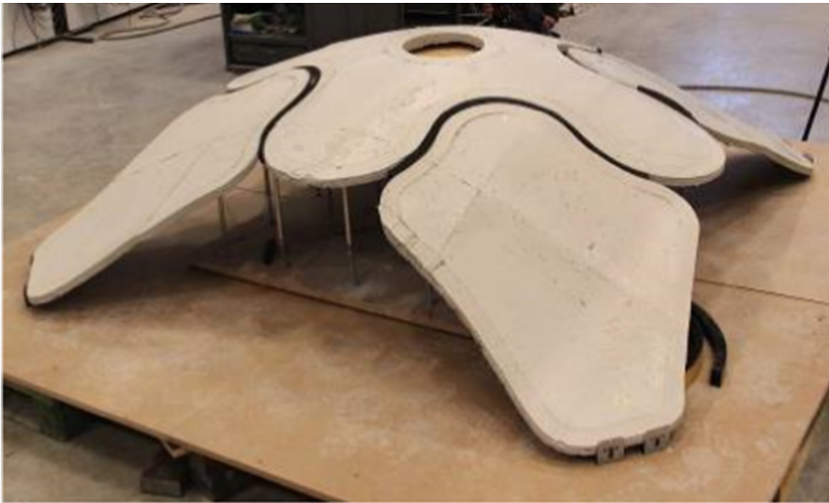
Figure 6.3: Contour printed and assembled shell, published in [18]
