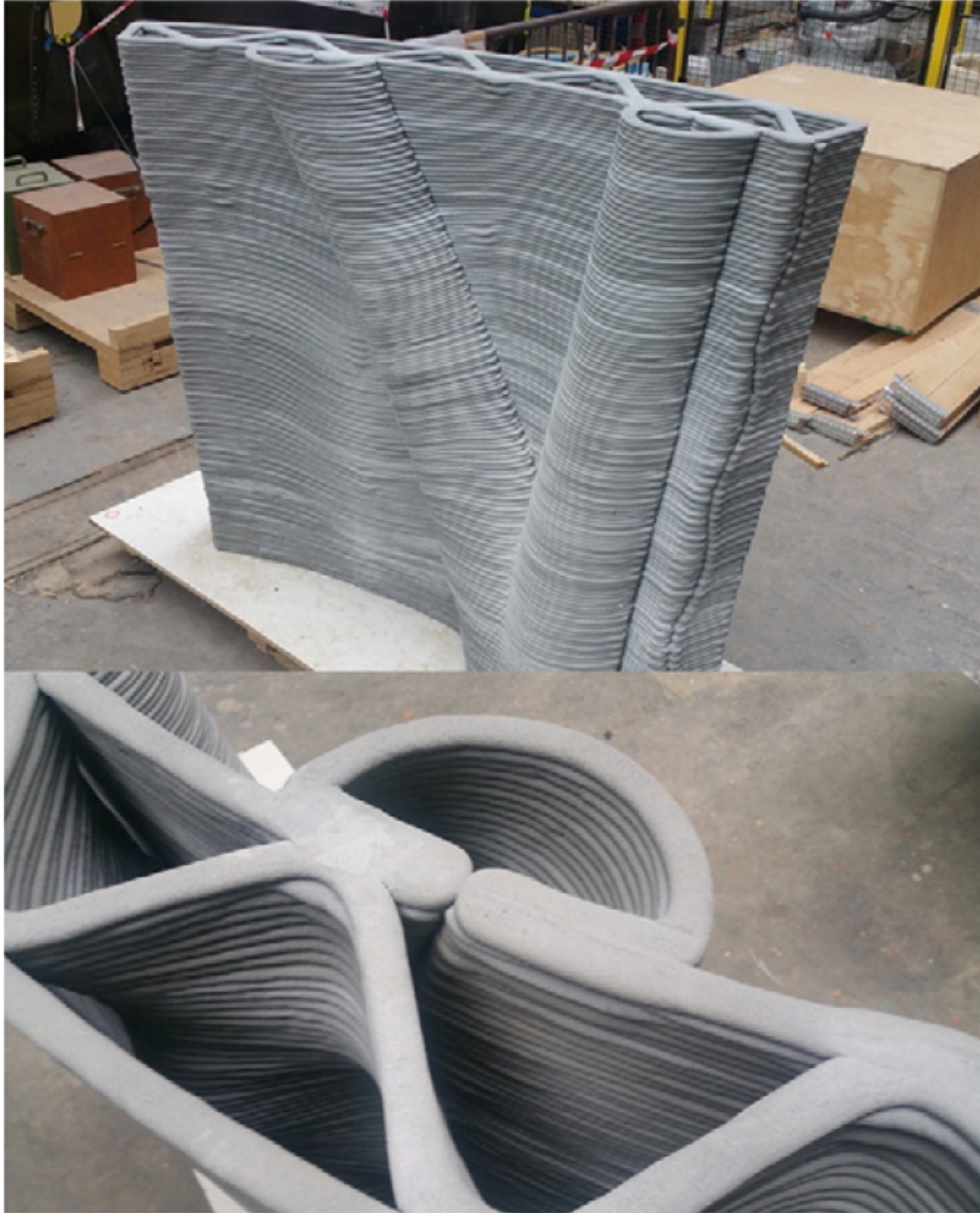
Figure 2.3: Doubly curved stiffened printed wall published in [31]
