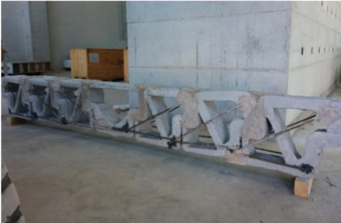
Figure 3.2: Externally reinforced beam (WASP, 2015)
