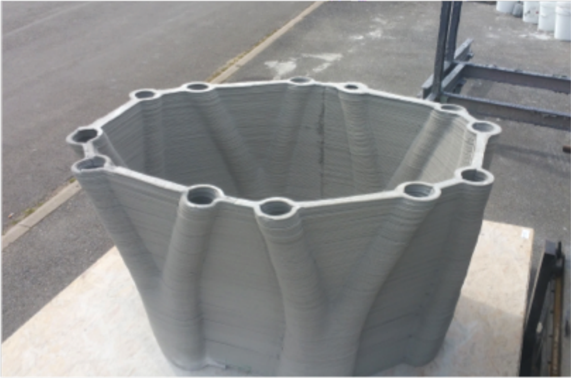
Figure 3.4: Mould for a space truss (XtreeE, 2016)
