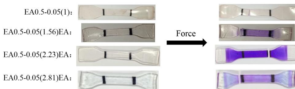
Figure 3.15: The mechanical response of the EA0.5-0.05 family group of elastomers
