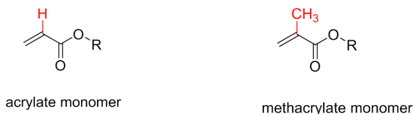
Figure 2.1: The difference between acrylate and methacrylate monomers
