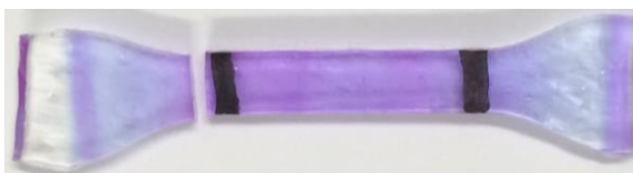
Figure 7.4 : Image of EA0.2-0.05(3.49)EA after the uniaxial tensile test
