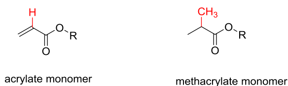
Figure 5.8: The molecular structure of acrylate and methacrylate monomers
