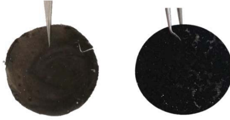
FIG. 3.11 - Photographs of the r-GO/PDMS composites before (left) and after (right) the thermal reduction.
