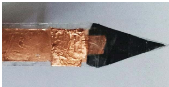
FIG. 5.2 - Photograph of the cantilever, top view.
