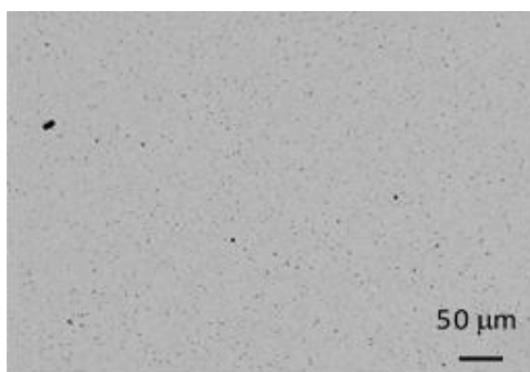
FIG. 4.2 - Microscopic picture of carbon black dispersion
