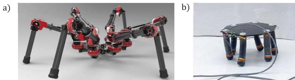
FIG. 1.1 - Comparison between two equivalent walking robots. a) HEBI Robotics based on mechanical actuators b) Electroactive robot [4].
