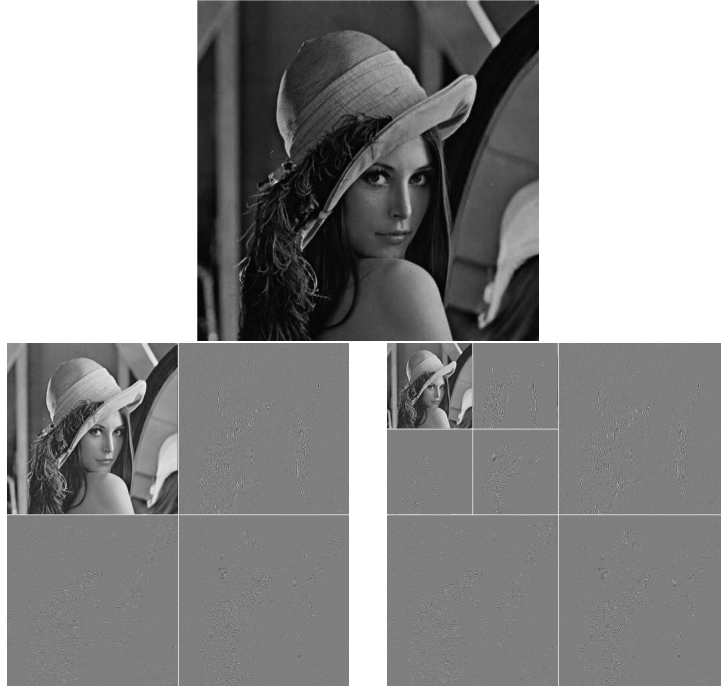
Figure 3.1 – Wavelet transform associated to Lena image for two decomposition levels. The size of the image is 512 by 512 pixels. The decomposition was performed using Daubechies wavelet with 12 vanishing moments. The approximation image corresponds to the subimage on the top left quarter. The other three subimages correspond to the projection of each approximation on a family of wavelets.
