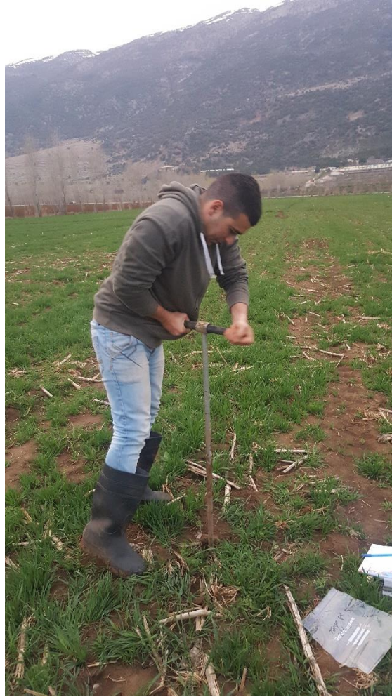
Figure 3 Soil sampling using a tube auger for W_s measurement. Photo taken in Ammiq, West Bekaa plain.
