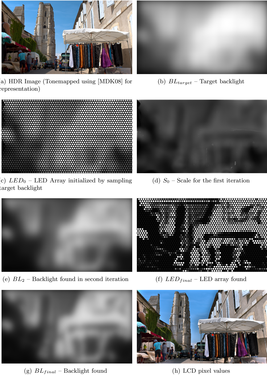
Figure 2.2 – Steps of the HDR image rendering algorithm for the HDR image Market3
