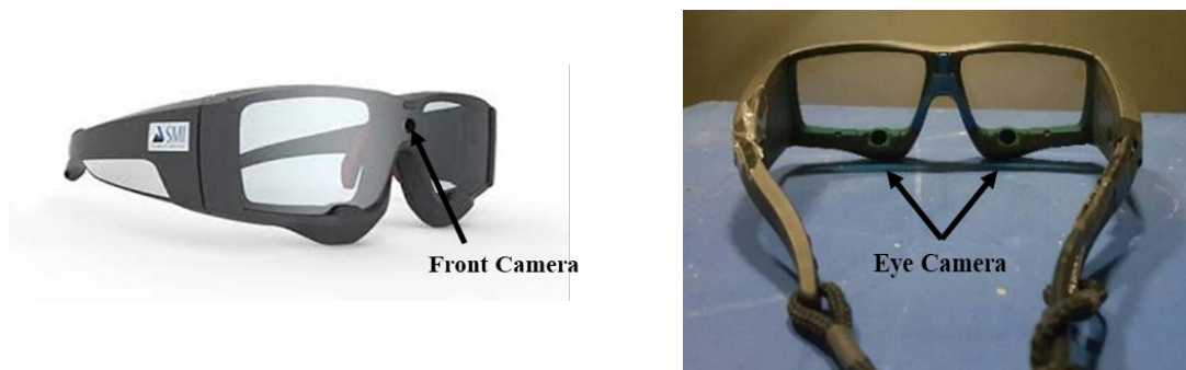
Figure 5.4 SMI eye tracking glasses used in this experiment.
