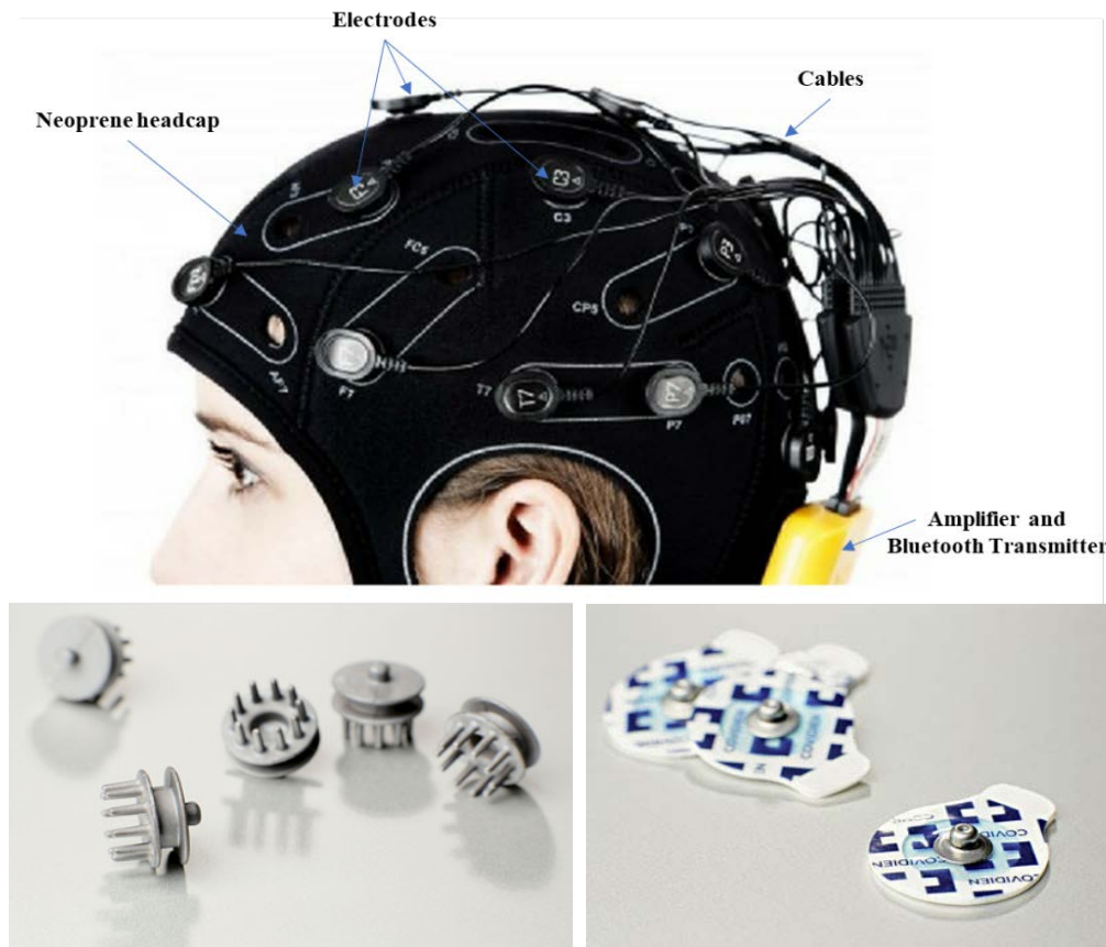
Figure 5.3 Top Image: Enobio 20 EEG wireless system, Bottom Left: Dry electrode, Bottom Right: Stickrode.
