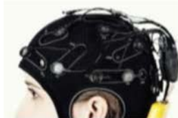
Figure 2: Neoprene headcap on subject's head with electrodes
