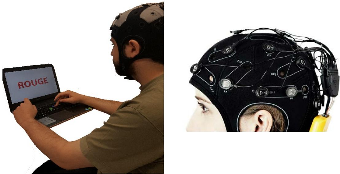
**Figure 4.3 Left Image:** Subject positioning during experiment, **Right Image:** Neoprene headcap used during the experiment.
