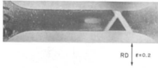
Figure 2.1 – Formation of a macroscopic shear band in a prestrained low carbon steel tensile test (Korbel and P. Martin (1988))
