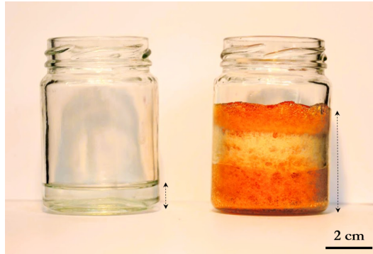
Figure 3.2 – Illustration of the volatile -induced porosity in the polyester resin. Left : initial monomer solution (dry content of 70 %wt). Right: resin obtained after curing. A huge foaming is observed due to the release of volatiles upon curing.
