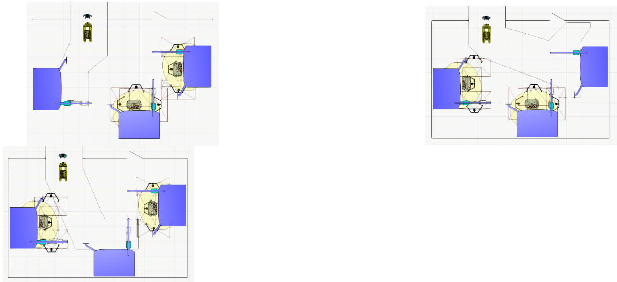
Figure 36: Pathway to access station 1, 2 and 3 with projector-based workspace monitoring systems as the safeguarding sensor and 100% POV robot speed
