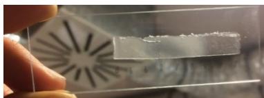
Figure 44: Picture of an inhomogeneous stripe of 1st generation of calibration sample
