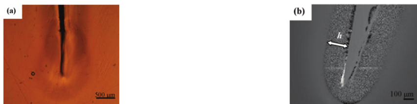
Figure 19: Visualization of the necked zone by optical microscopy (a) and high-low image (b)
