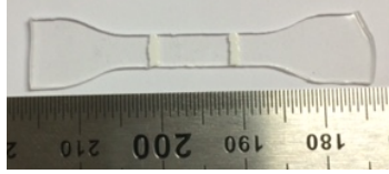
Figure 8: Picture of a sample used for uniaxiale extension test
